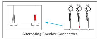
The subwoofer can be connected to any connector on the harness. However, it is recommended that it be placed as close as possible to the center of the speaker array.
