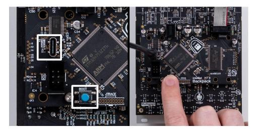
Plug a USB-C cable between the module's USB-C port and a computer.
