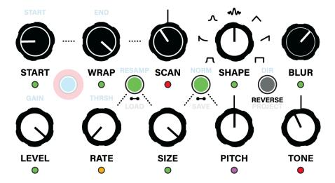
The three **BLACK KNOBS** on the top-left of the panel are the **Position Controls**. They determine where grains are generated from in the Sample or Looping Recorder (for Live Sounds).
