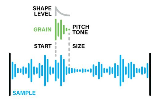
As mentioned near the start of this manual, grains are just small fragments of audio from a larger audio sample.
