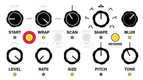
When a Mod Page is active, the **10 KNOBS** act as attenuverters for their given parameters.
