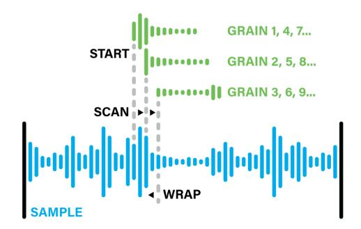
In the diagram above, you'll see the application of **START**, **SCAN**, and **WRAP**. In this simplified example, grains are generated from a small area of the sample or Live Memory at an arbitrary **RATE** while the Sound is playing. Restarting the playback of a Sound will reset the scanned position to **START**.
