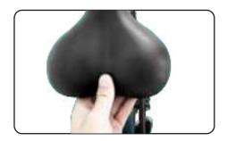
Adjust the seat and the head of the seat to be parallel with the top tube.
