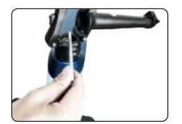
Use Allen Wrench to loosen the center screw.
