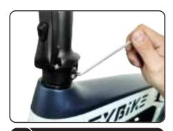
Fold the tube back and lock the latch. Tighten the screws on the side.
