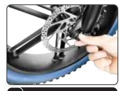
Make sure the position of each part is correct, tighten the nut. Then install the front fork cover.
