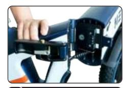
Unlock the latch. Unfold the rear wheel/ section and hold your e-bike upright with the kickstand.
