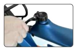
Open the quick-release lever by swinging the lever open and outward fully.
