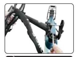
Adjust the handlebar and tighten the screw to fix the headtube.
