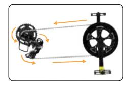
Check the chain alignment. Rotate the right pedal and crank toward the back of the bike as though pedaling backward. Watch the chain and ensure the chain runs through the drive train (the rear cog, chain tensioner, and around the front chainring) smoothly.
