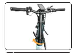
With the tube upright, turn the bike head clockwise 180 degrees horizontally.
