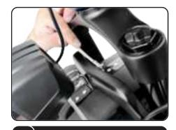
Attach the front fender and the headlight onto the bike frame and align the holes.
