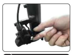
Remove 1 the black retainer in the brake caliper and 2) the front fork retainer lever.
