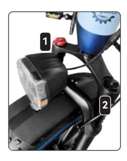
The preload adjustment knob (2), located on the top of the left side of the suspensionfork. To soften the ride, subtract resistance by turning the preload adjustment knob counterclockwise, in the direction of the small "-" on the knob. To make the suspension stiffer when going over bumps, add resistance by turning the preload adjustment knob clockwise, in the direction of the small "+" on the knob.
