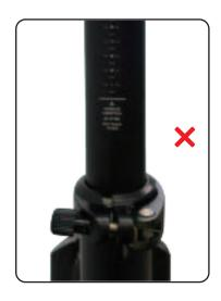
(2) Before using the bike, always check to ensure all latches, levers, and quick releases are properly secured and undamaged. Check that they are correctly secured before every ride and after every time the bike is left unsupervised, even for a short time. Otherwise, the handlebar stem and/or seatpost may come loose and can result in loss of control, damage to the bike, property, serious injury, and/or death.
