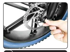
Make sure the position of each part is correct, tighten the nut. Then install the front fork
