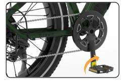
Locate the right/left side pedal, which has the "R"/"L" sticker attached.
