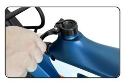
Open the quick-release lever by swinging the lever open and outward fully.
