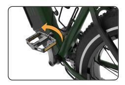
Thread the right pedal onto the right crank gently by hand, turning clockwise. Then tighten the pedal with Allen Wrench.
