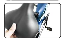
Move the seat up and down by sliding the seatpost in or out of the seat tube. DO NOT raise the seatpost beyond the minimum insertion marking etched into the seatpost
