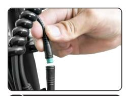
7 The arrows of the two interfaces are aligned and installed to ensure the straight line alignment.
