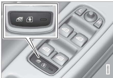
Driver's door control panel
