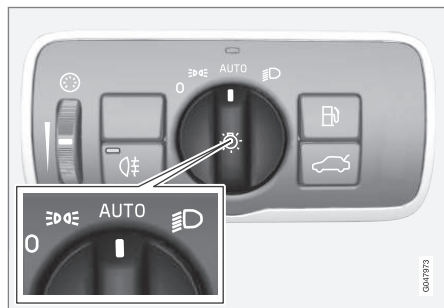
Headlight switch in the AUTO position
