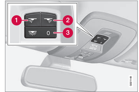
Light switches, front roof lighting
