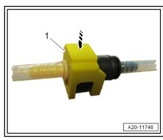
Secure retaining clip -1- on plug-in connector -3- with cable tie
