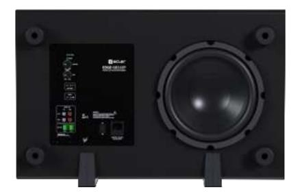
The EDGE-SB110P has a balanced Euroblock audio input, a balanced Euroblock stack audio output, and two unbalanced RCA audio inputs, labelled left and right. You can send them a mono or stereo line-level signal: the SB110P internally works on mono signals and, therefore, adds L and R input signals to obtain a valid signal to work on. You can link a second EDGE-SB110P unit or other auxiliary equipment using L and R STACK outputs, also on RCA connectors.
