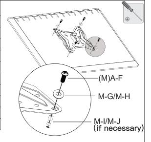
First, make sure the diameter of the bolt ((M)A - F) fits your TV. Then, please see the diagram above. You will need to thread the bolt into the TV using the correct washer (M-G/M-H) and spacer (M-I/M-J) if necessary. Please make sure the monitor bracket is vertically centered.
