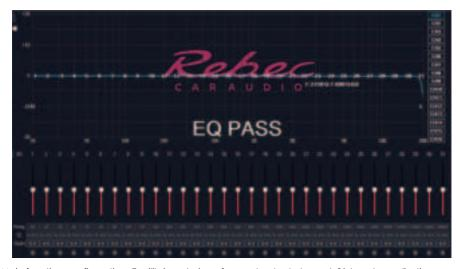
Main function configuration: Equilibrium design of current output channel, 31-band equalization adjustable: frequency, Q value (response bandwidth) and gain (increasing or decreasing the frequency response amplitude near the frequency point).
