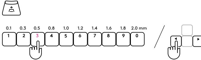
Press any alphabet key to test the current sensitivity setting. When pressed and released, the key's light turns blue when actuated and magenta when it resets.
