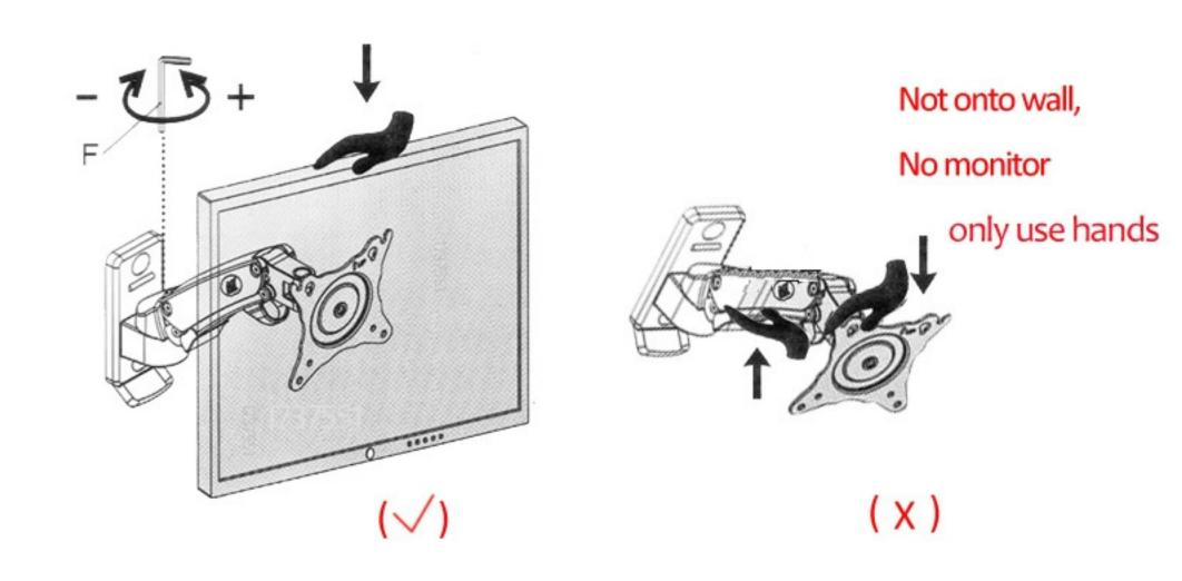
2. Question: the torque adjust hole is not able to reach Answer: first, finish the instal and attach monitor onto the mount, second, press the arm down, then the hole will come out
