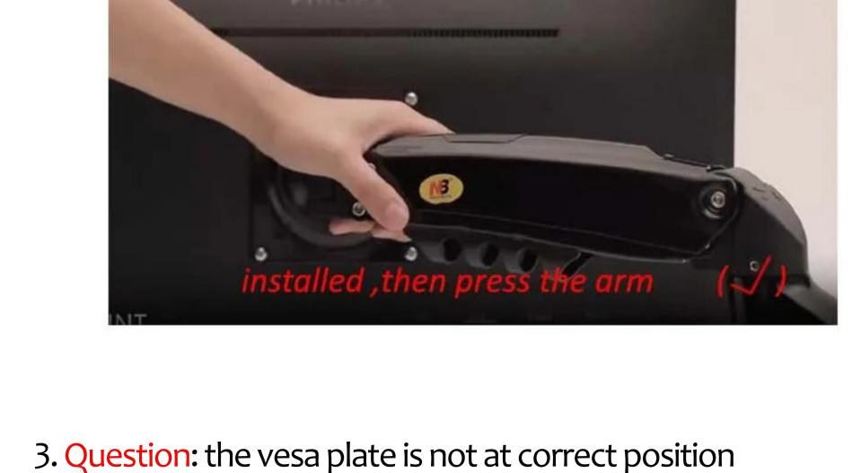
Answer: the VESA plate could rotate by 360°, catch the screen and rotate
