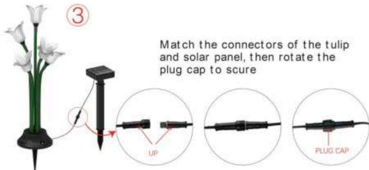
Match the connectors of the tulip and solar panel, then rotate the plug cap to secure
