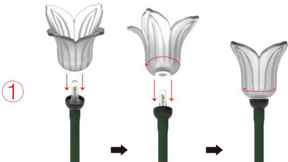
Align the tulip with the interface and rotate to secure
