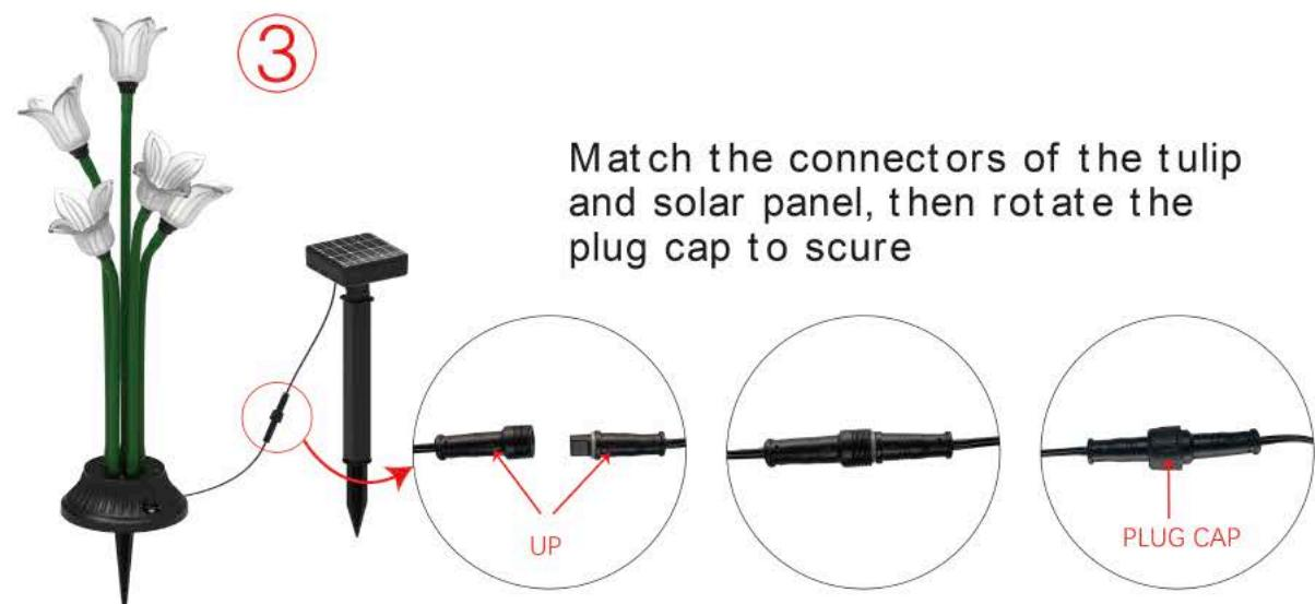
Match the connectors of the tulip and solar panel, then rotate the plug cap to secure
