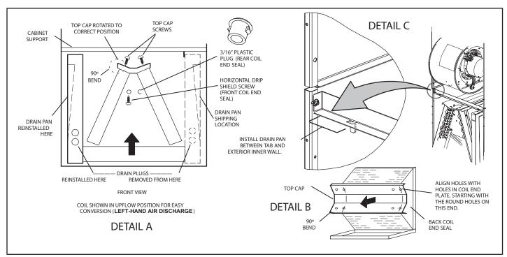
FIGURE 5. Field Modification for Left-Hand Discharge
