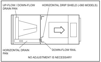
FIGURE 2. Right-Hand Discharge Configuration
