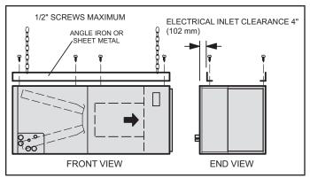
FIGURE 3. Suspending Horizontal Unit
