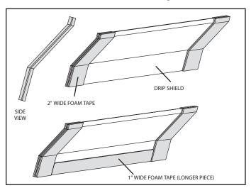
FIGURE 7. Applying Foam Tape to Drip Shield
