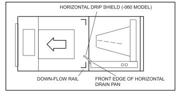
FIGURE 4. Left-Hand Discharge Configuration
