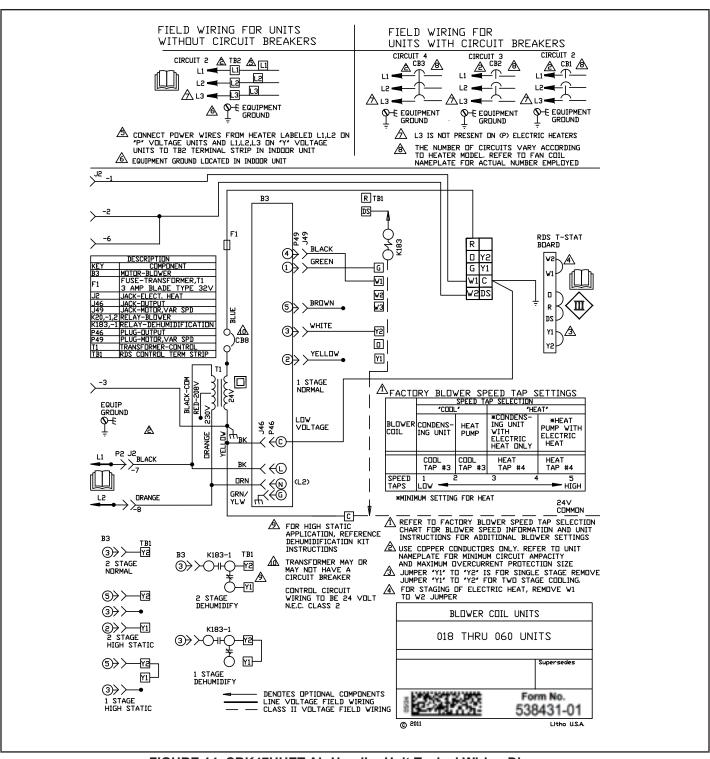
FIGURE 14. CBK47UHET Air Handler Unit Typical Wiring Diagram
