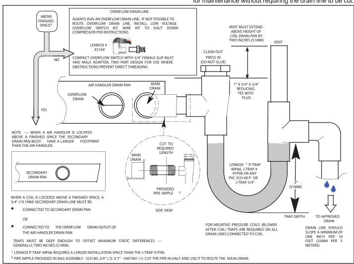
FIGURE 13. Typical Main and Overflow Drain Installations
