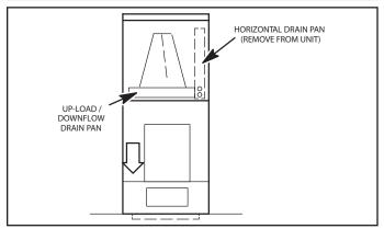
FIGURE 6. Downflow Discharge Position
