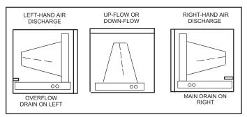
FIGURE 12. Main and Overflow Drain Locations
