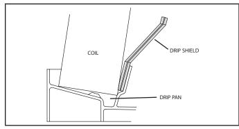
FIGURE 8. Downflow Drip Shields
