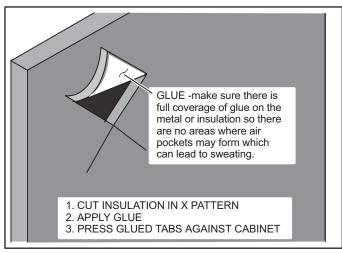
FIGURE 17. Repairing Insulation
