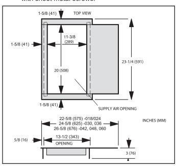
FIGURE 10. Downflow Combustible Base Dimensions
