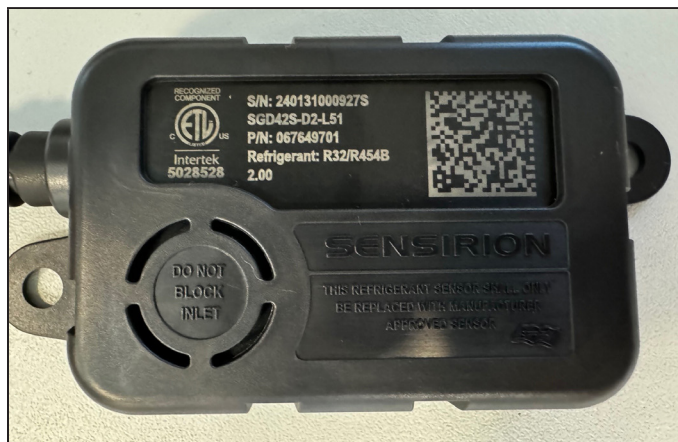
FIGURE 18. Example of Clear, Unobstructed Sensor Inlet
