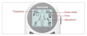
(5) Repeat press MENU again to set up waveform, frequency,pulse width by pressing CH2  $\blacktriangle/\blacktriangledown$ .
