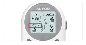
(6) If you want to select manual modes of EMS, press P to adjust program to P22 and just repeat above steps of P11 to get started. Besides, P22 has 4 more adjustable parameters, they are rise time, action time, fall time and rest time.
