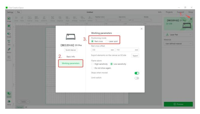
If the **Laser spot** is selected as the positioning mode, you have to click **Process > Enable** every time for the laser to emerge.
