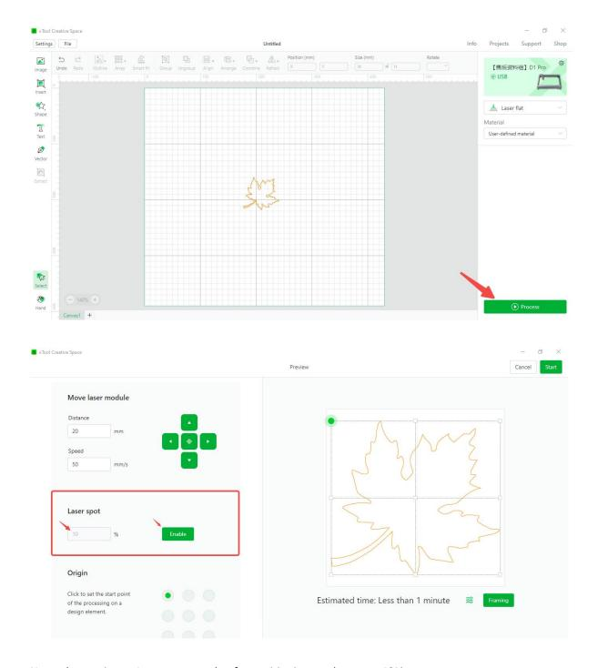
Note: the maximum Laser power value for positioning can be set to 10%.
