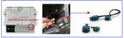
2)If your car's original antenna interface is a separated dual hole, as shown in the middle picture below, we also recommend purchasing a dual-hole antenna to ensure the normal operation of the antenna.
