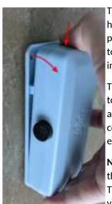
To "clip" a Sensor into a Backplate align the hook at the bottom of the Sensor with the pocket on the Backplate, then rotate in towards the Backplate until the Sensor locks into place (see right).
