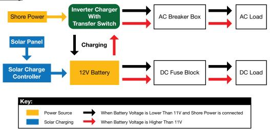
When set to DC priority, the inverter will utilize the battery bank for electricity. When battery voltage gets too low, it will automatically switch to shore power. Charging can be turned off by setting battery switch to 0. (See Page 10)
