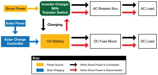
When set to AC priority, you will draw from shore power and not the battery bank. When not connected to shore power, DC power from the battery bank/solar will be converted into AC.
