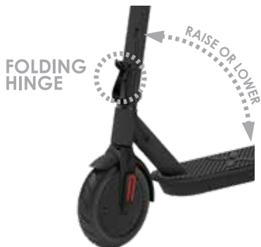
RELEASE FOLDING HINGE TO FOLD STEERING COLUMN
