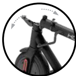
RELEASE FOLDING HINGE TO FOLD STEERING COLUMN
