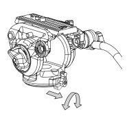
You can change the position by turning the pan lock knob while pulling it towards you. Please adjust it to a position that does not interfere with the tripod.
