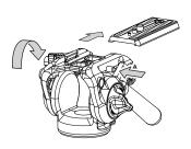
Turn the shoe lock knob in the direction of the arrow to loosen it, and then press the release button to remove the quick shoe. The quick shoe can only be removed from the front side (pan handle side).
