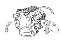
Loosening the tilt lock knob allows you to tilt the equipment upwards or downwards.
