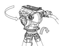
You can remove the tripod head by tightening the pan lock knob on the head and rotating the head counterclockwise.
