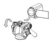
Attach the quick shoe with the equipment attached to it to the tripod head from the front. Tighten the shoe lock knob to secure it in place at a well-balanced position. The quick shoe can only be attached from the front.
