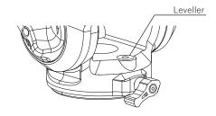
Using the leveller on the camera head can be used as a guide for leveling when taking photos. The leveller for the tripod is a guide for level adjustment. The accuracy is different from the leveller built into the camera.
