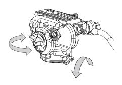
Loosen the pan lock knob to pan your equipment left and right.
