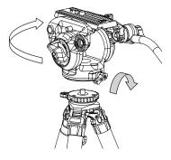
Tighten the pan lock knob on the head, align the screws on the tripod and head, and turn the head clockwise to screw it in tightly.
