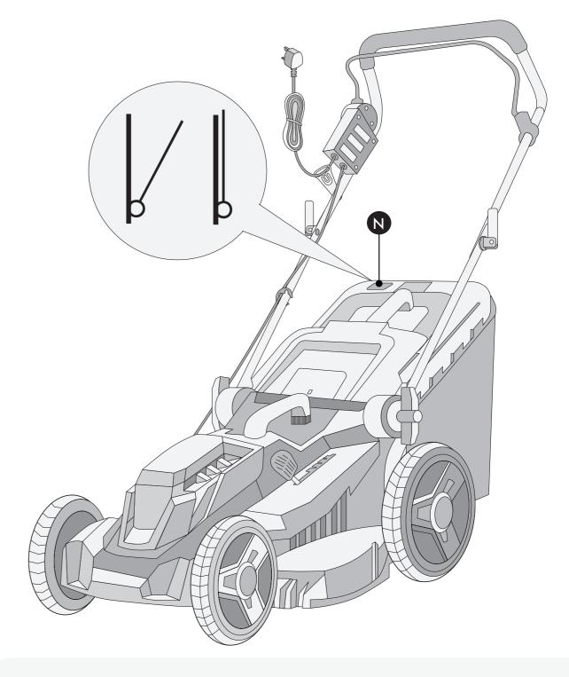
The GRASS INDICATOR (N) is equipped with a hatch that indicates the filling during operation.
