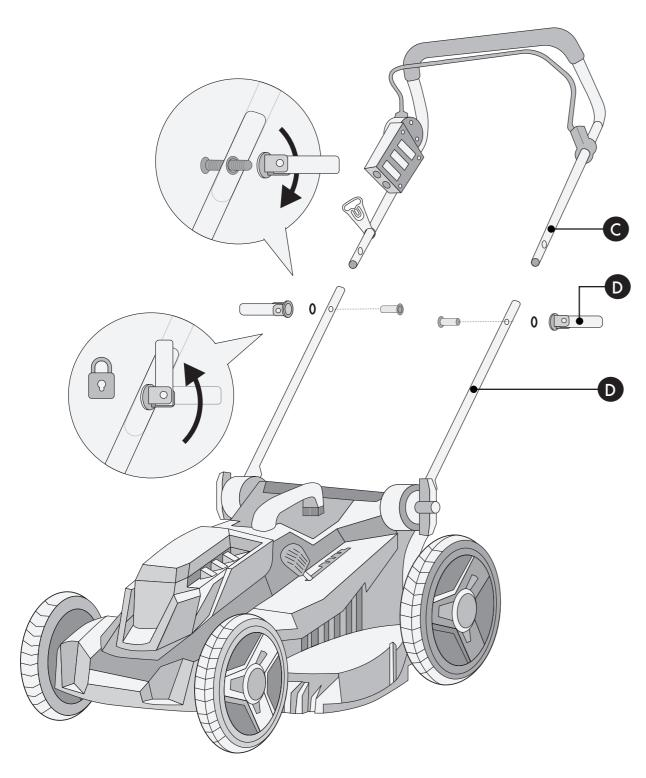
Connect the LOWER SUPPORT BARS (D) with the UPPER SUPPORT BARS (C) using the WING NUTS (F)
