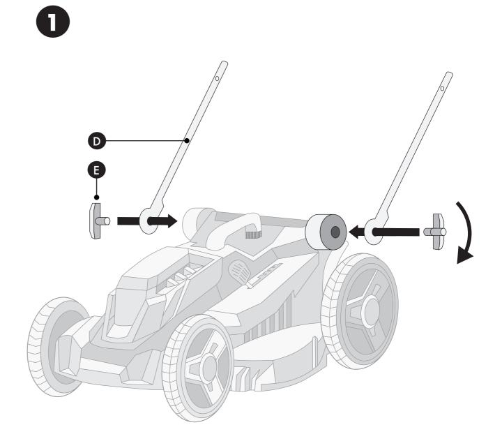
The LOWER SUPPORT BARS (D) are fixed on the main unit through the engagement of the teeth on the LOCKING KNOB ASSEMBLY (E). Rotate to lock.
