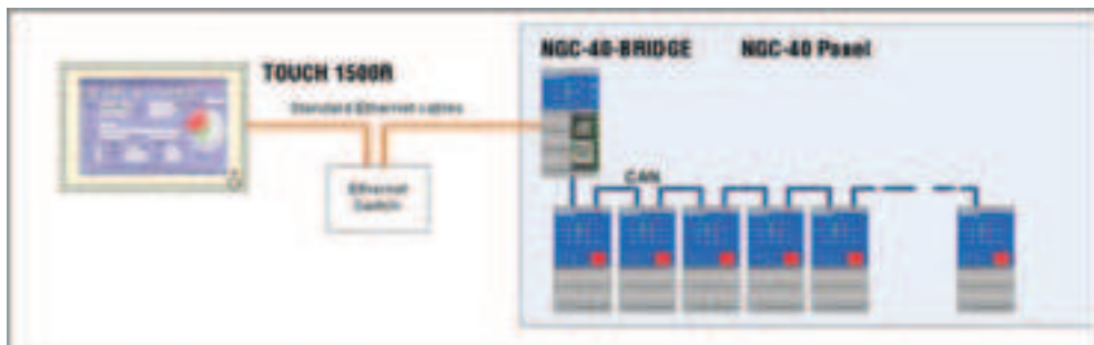
Figure A.2 Connecting to NGC-40-BRIDGE using Ethernet switch and standard Ethernet cable
