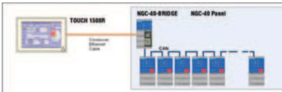
Figure A.1 Connecting directly to NGC-40-BRIDGE using Ethernet crossover cable
