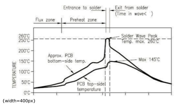
Recommended soldering temperature:
