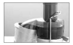
Place both hands on either side of the safety locking arm and pull back and lift over the grooves on either side of the juicing cover.
