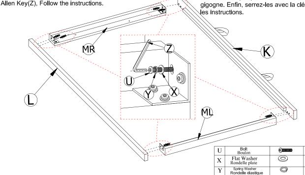
Step 10: Install the trundle frame in step 8 and step 9 together with bolt (R), flat washer (RS) and spring washer (XY). Finally, tighten them with Allen Key(Z), Follow the instructions. Note: It is recommended to turn them upside down for easy installation
