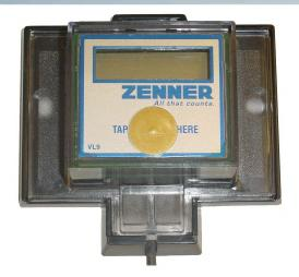
The VL-9M electronics and battery are environmentally sealed and suitable for outdoor installation, the wire terminals are not sealed for moisture. The unit should not be installed in locations below grade or in a submersible environment.
