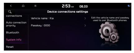
The passykey is a 4-digit authentication code used for a Bluetooth connection between the mobile phone and car system. The defauly passkey is set to 0000.
