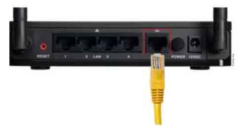
STEP 3 Connect one end of a different Ethernet cable to one of the LAN (Ethernet) ports on the back of the unit. (In this example, the LAN 1 port is used.) Connect the other end to an Ethernet port on the PC that you will use to run the web-based Setup Wizard and Device Manager.
