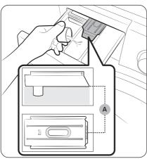
3. Apply fabric softener to the **softener** compartment. Do not exceed the max line (A). Softener is dispensed into the wash during the final rinse.
