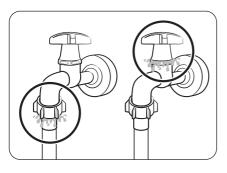
Open the water tap and check if there are any leaks around the connection areas. If there are water leaks, repeat the steps above.
