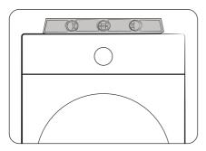
2. Level the washing machine by manually adjusting the levelling feet.
