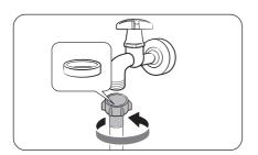
1. Connect the water hose to the water tap, and then turn the connector clockwise as shown.
