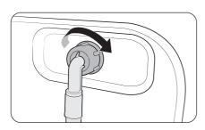
**2.** Connect the other end of the water hose to the inlet valve on the back of the washing machine. Turn the hose clockwise to tighten.
