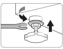
3. When levelling is complete, tighten the nuts using the spanner.
