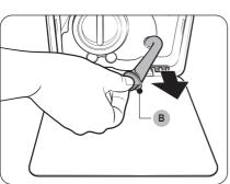
**3.** Put an empty, spacious container around the cover, and stretch the emergency drain tube to the container while holding the **tube cap (B)**.
