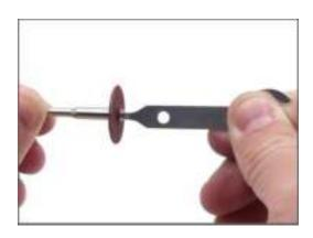
Unscrew the mandrel screws and install 3 or more discs of sandpaper
