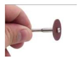
Insert the installed sandpaper device into the chuck and tighten with the wrench. Then tighten the screws on the mandrel head with the wrench.
