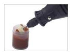
Dip the felt wheel into the polishing paste and rotate it at a low speed ,then apply the felt wheel to the polishing project.
