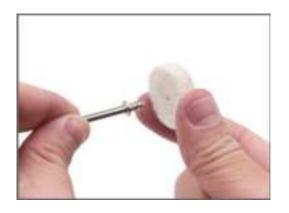
Insert the mandrel into the felt wheel
