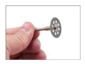
Install the mounted cutting disc in the chuck, and fasten the chuck and the cutting disc screw with the wrench
