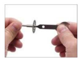
Unscrew the head screw of the mandrel and attach the cutting disc
