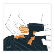
Locate the locking pin and press in points shown to remove.
