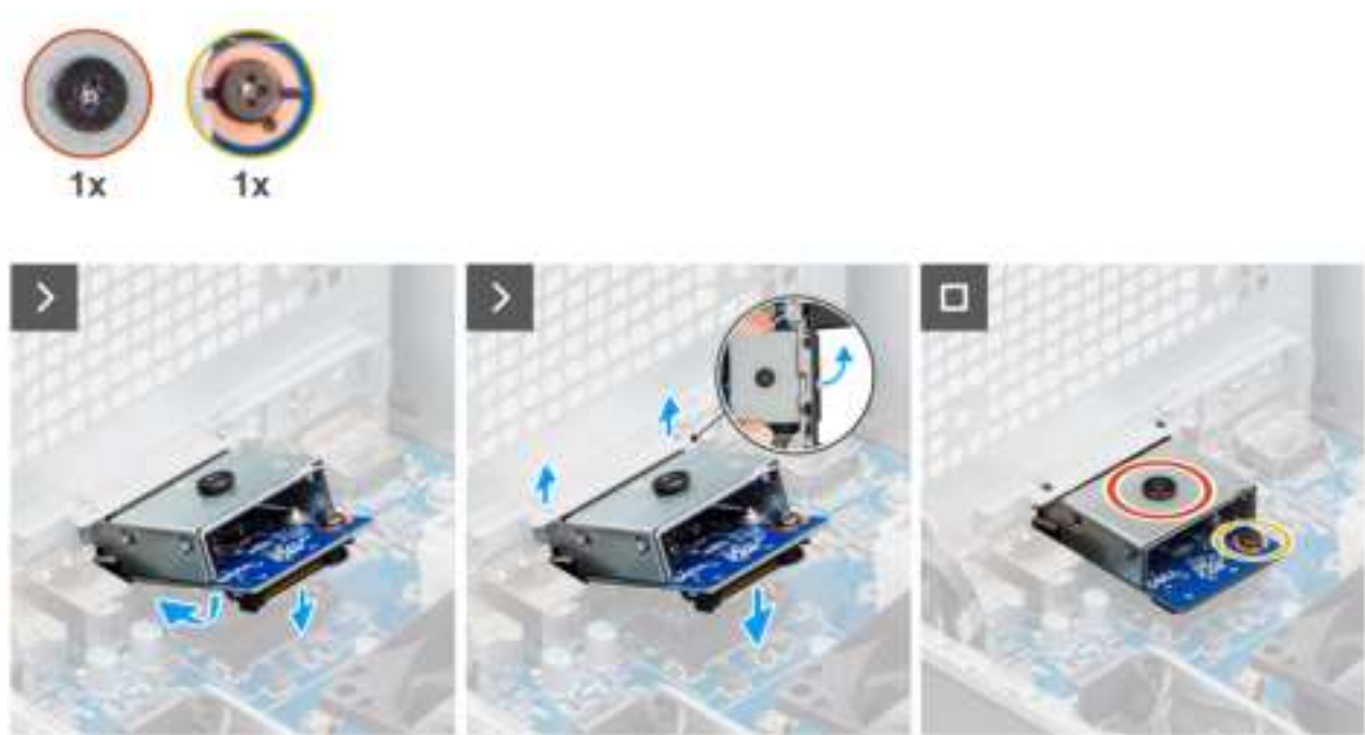
Figure 87. Installing the optional VGA module
