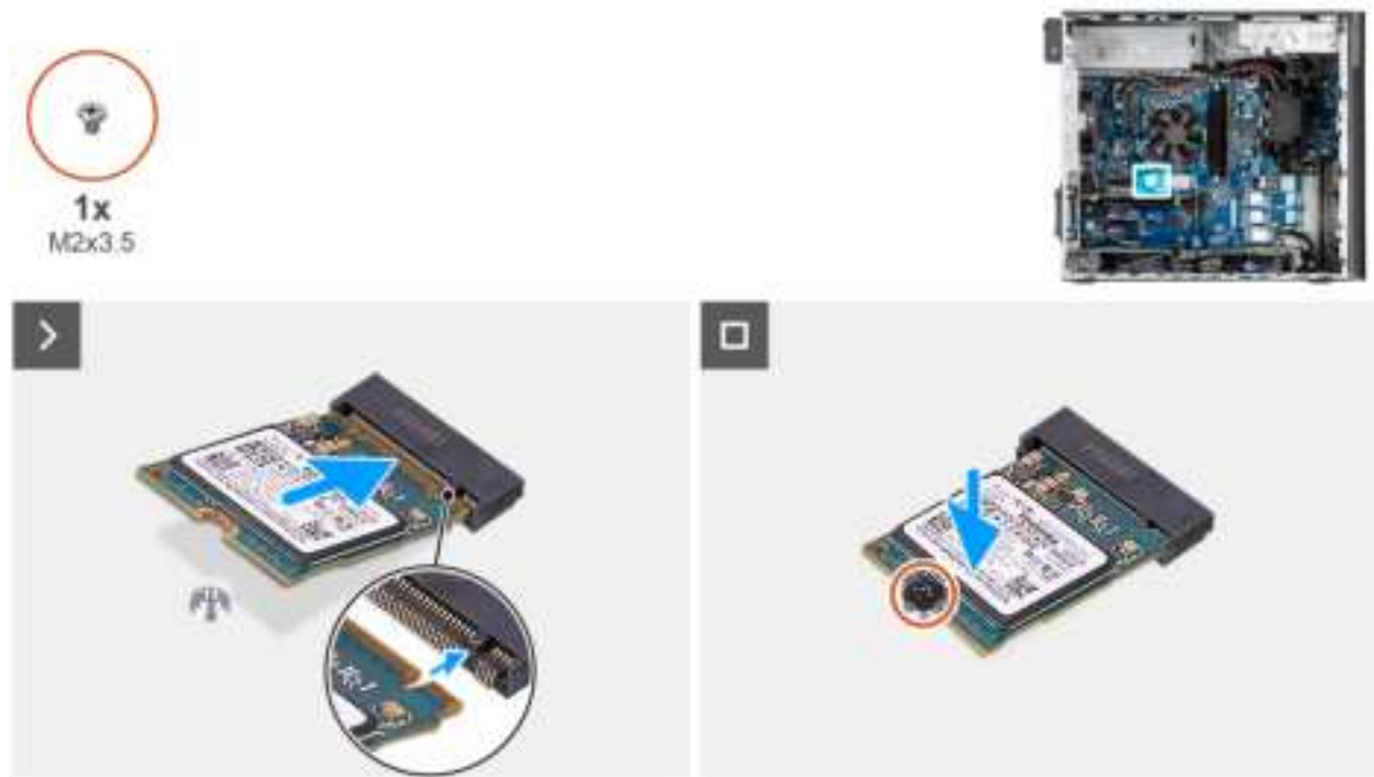
Figure 32. Installing the M.2 2230 PCIe solid state drive
