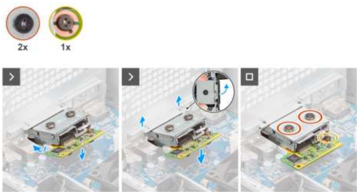
Figure 75. Installing the optional 5GbE Optical module
