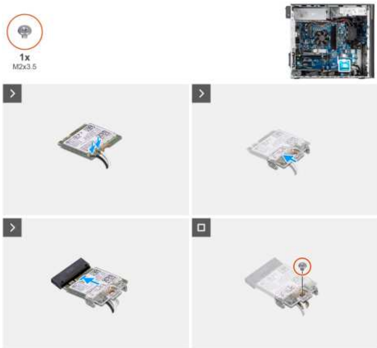
Figure 42. Installing the wireless card
