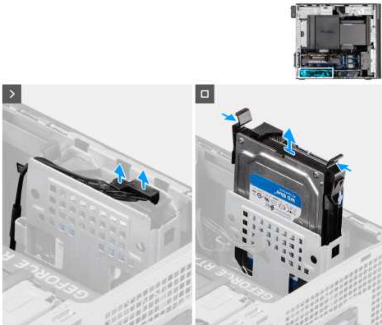
Figure 26. Removing the 3.5-inch hard drive assembly (Bay-2)
