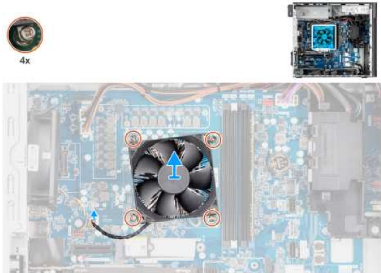
Figure 61. Removing the processor fan and 65 W heat-sink assembly
