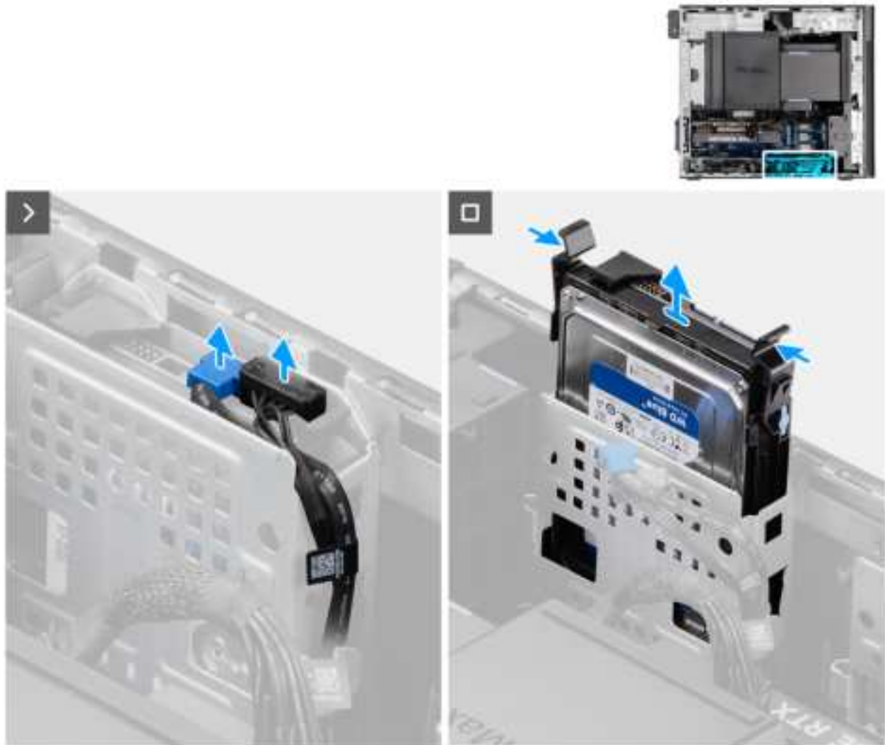
Figure 25. Removing the 3.5-inch hard drive assembly from Bay 1
