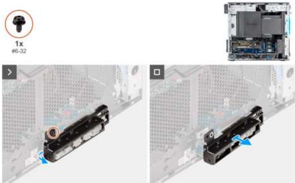
Figure 19. Removing the front I/O bracket
