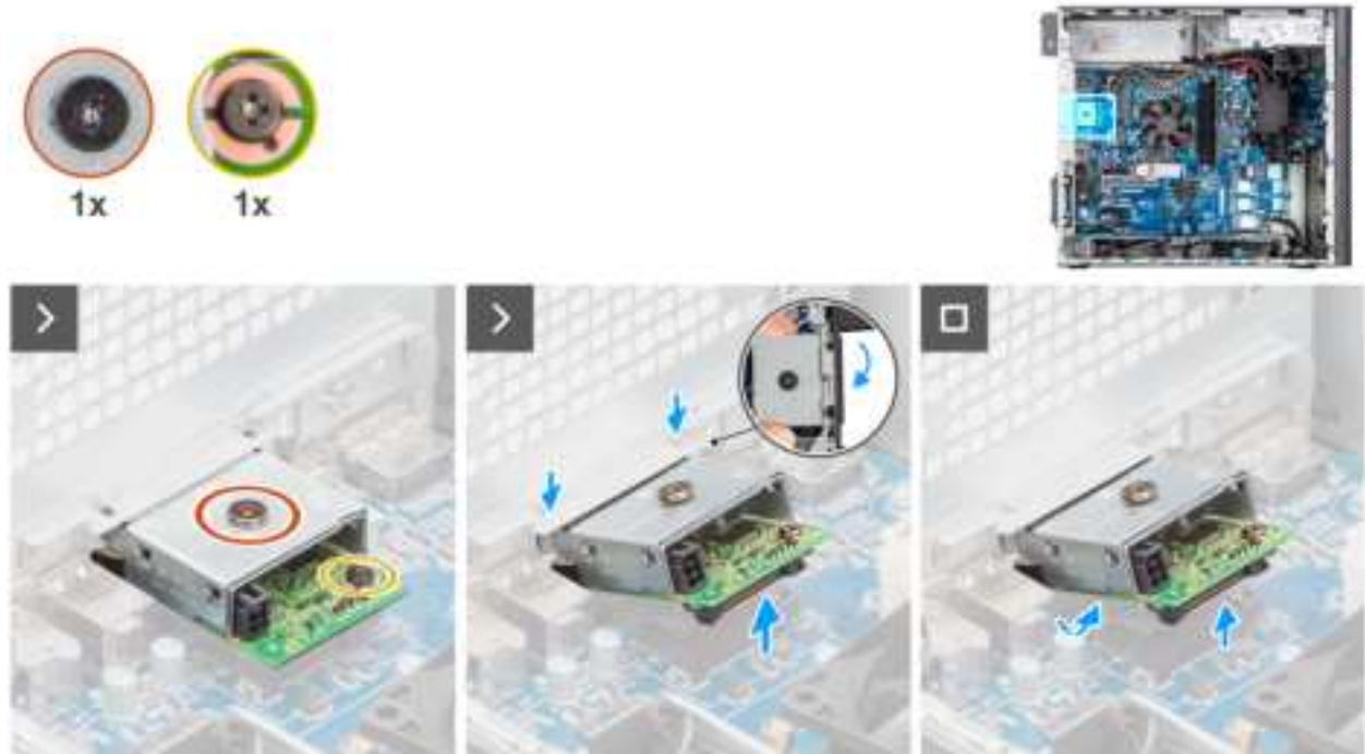
Figure 82. Removing the optional USB module
