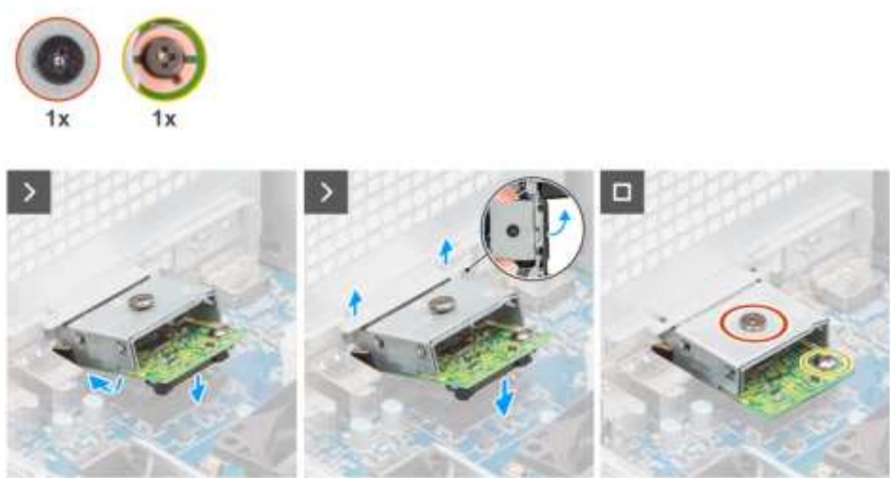
Figure 69. Installing the optional DisplayPort module
