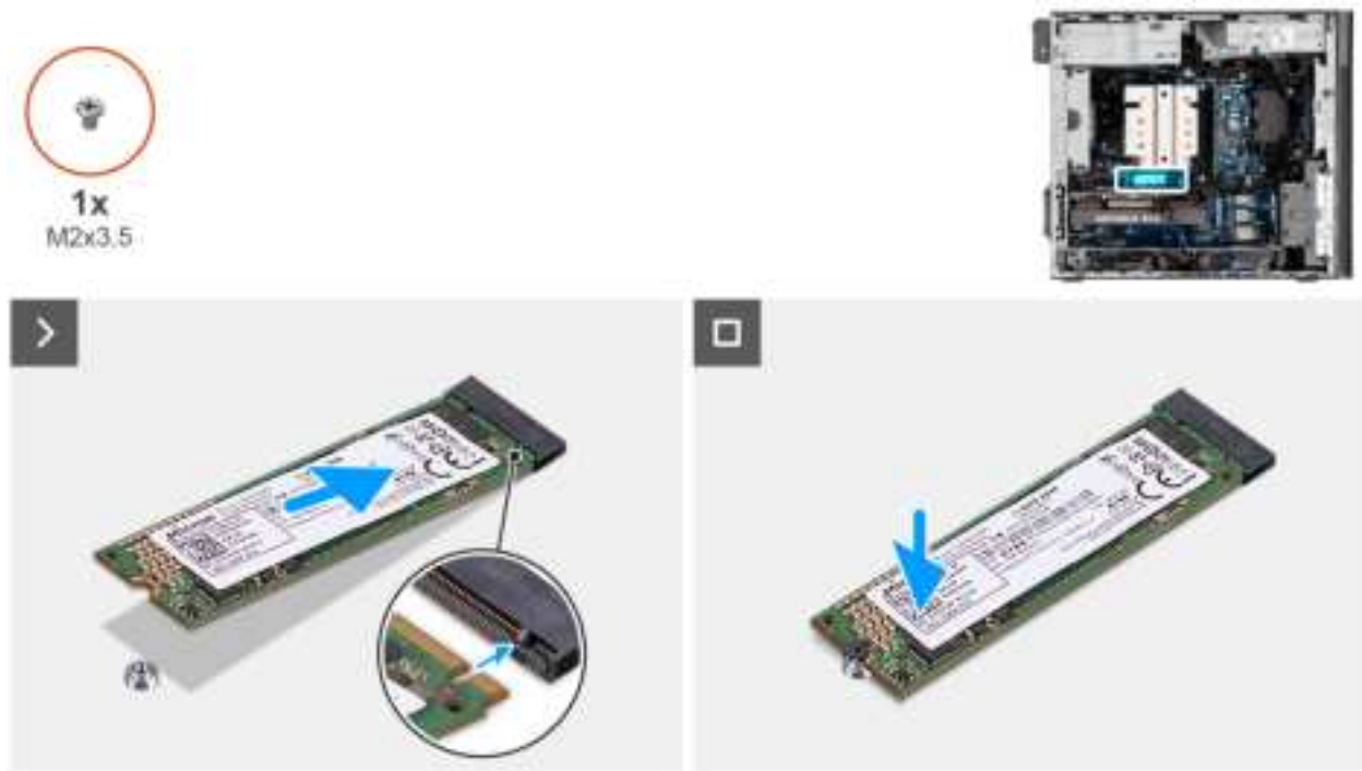
Figure 34. Installing the M.2 2280 PCIe solid state drive
