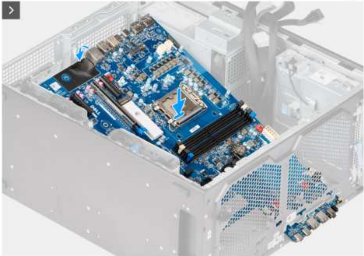
Figure 94. Installing the system board
