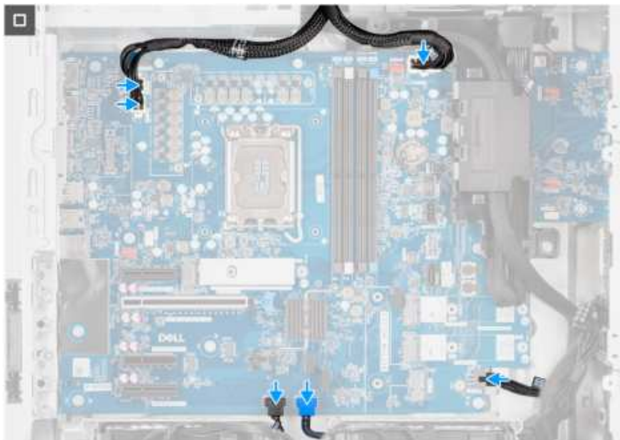
Figure 97. Installing the system board
