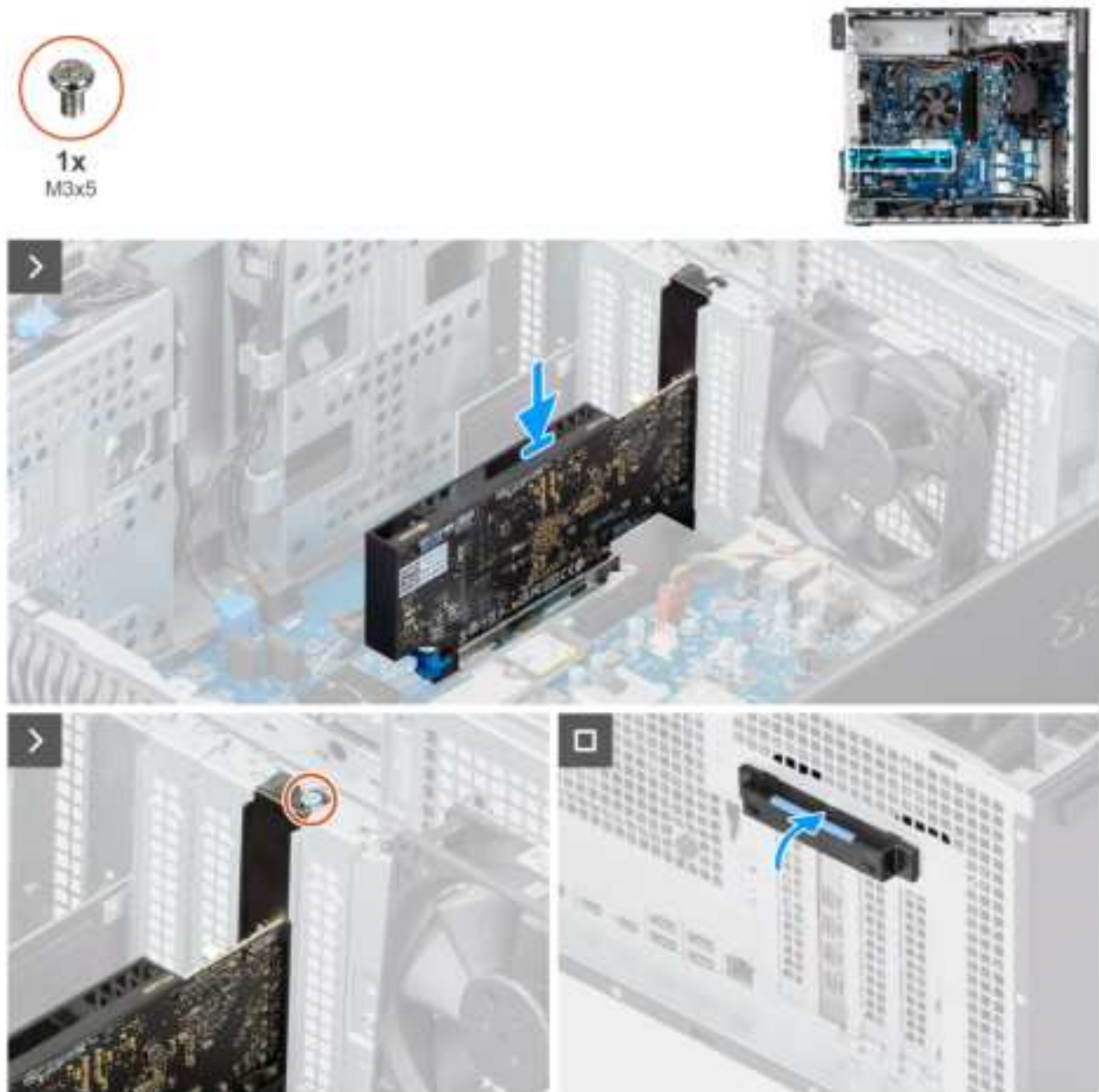
Figure 38. Installing the graphics card
