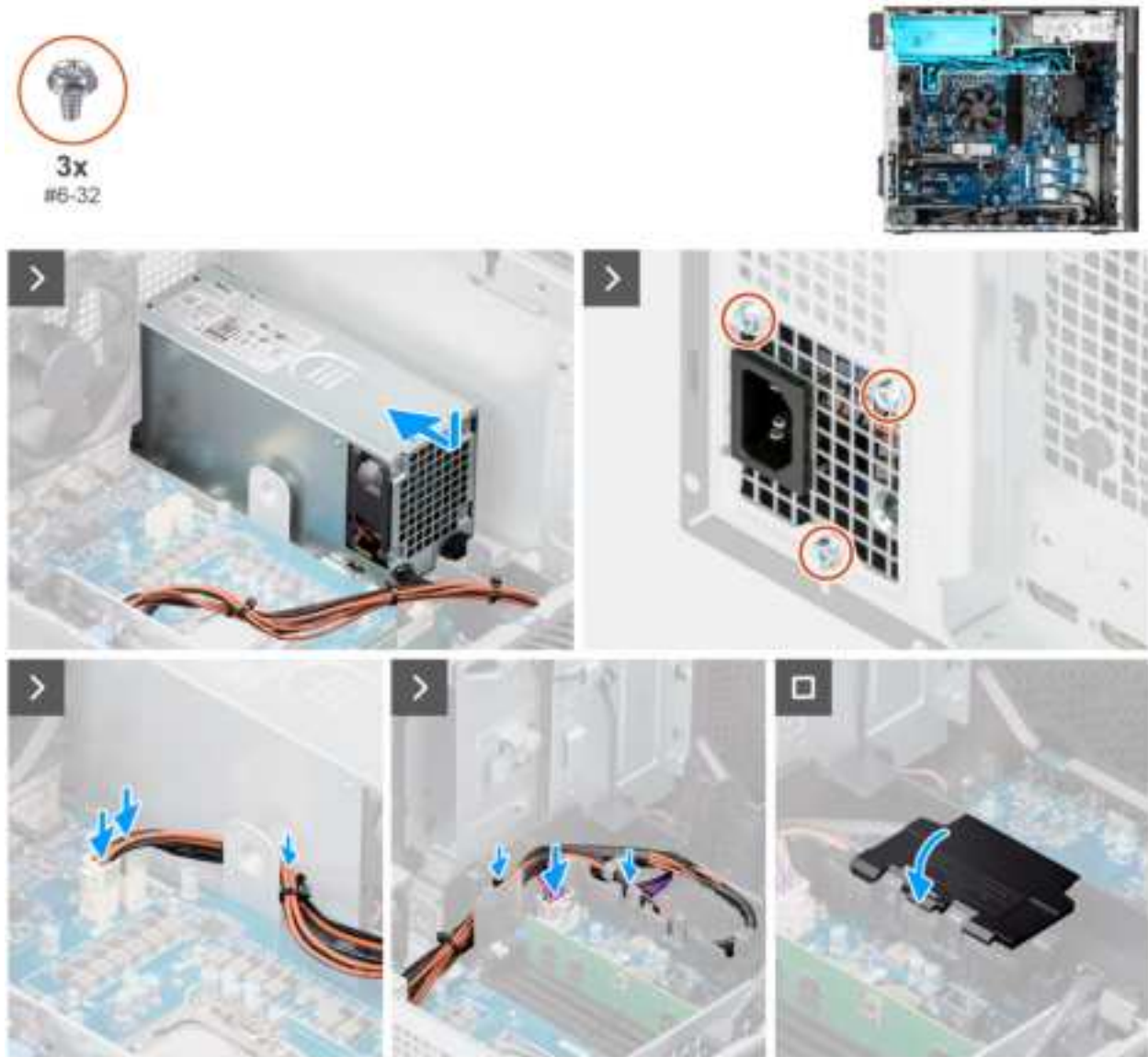
Figure 58. Installing the 360 W power-supply unit
