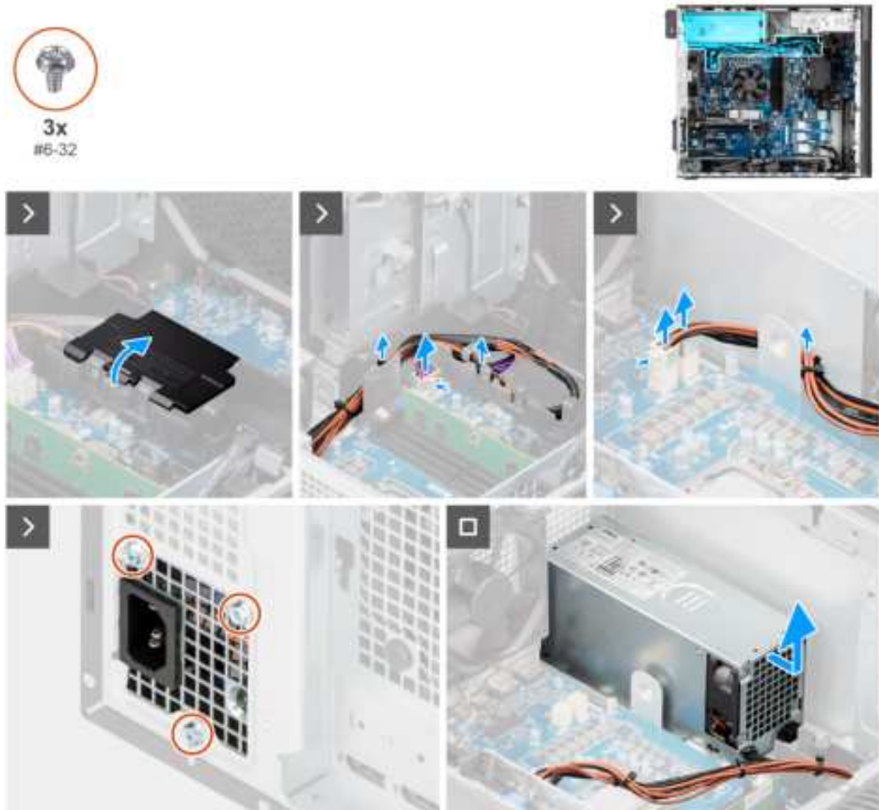
Figure 57. Removing the 360 W power-supply unit
