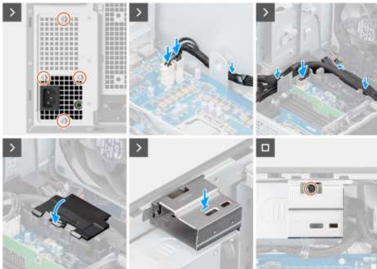
Figure 56. Installing the 1500 W power-supply unit
