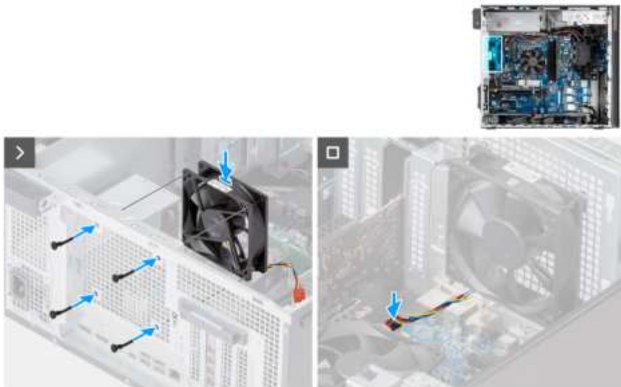
Figure 50. Installing the rear fan for 360 W PSU computers
