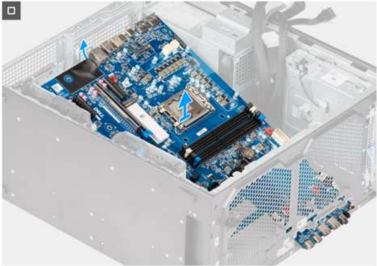
Figure 92. Removing the system board
