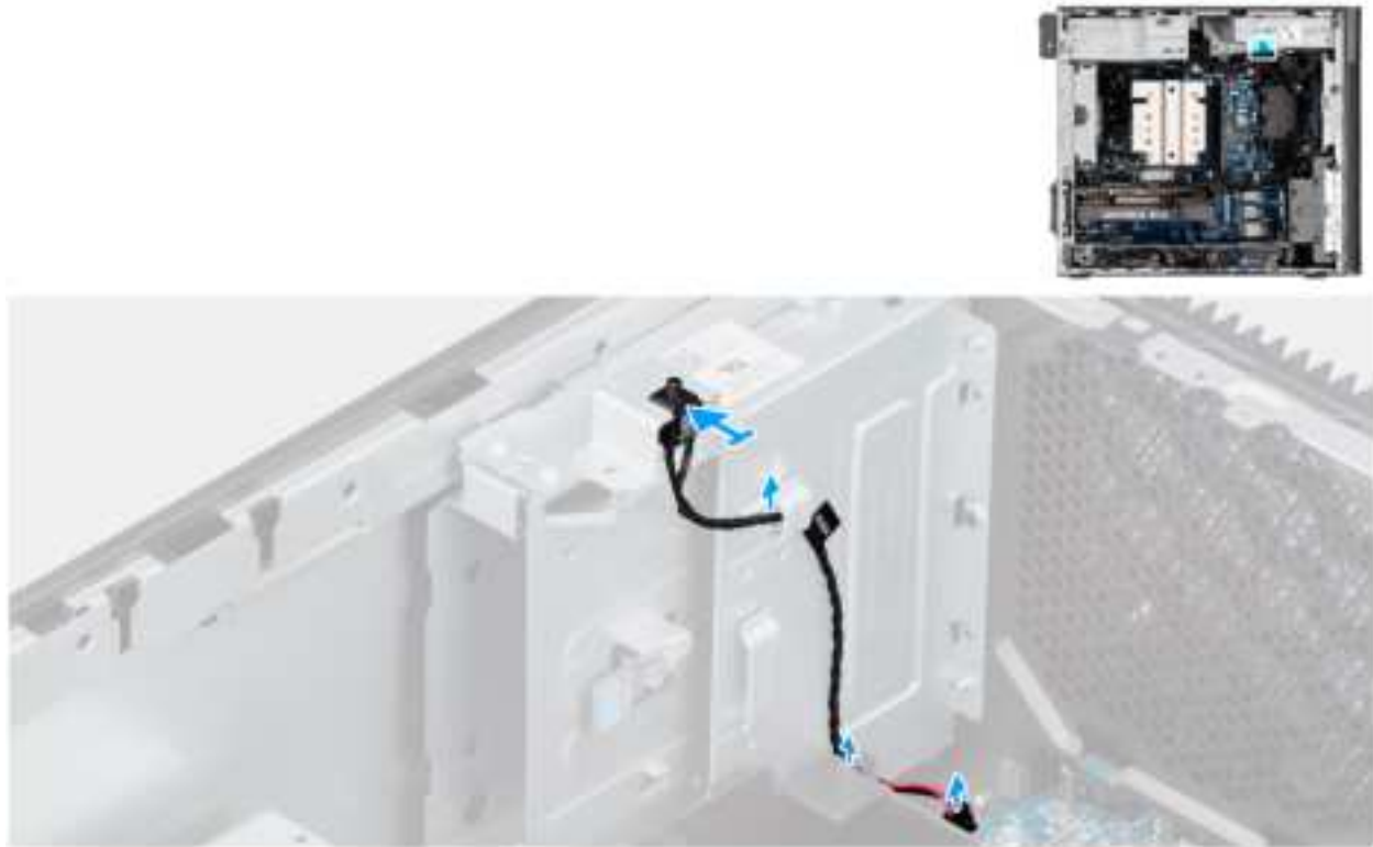
Figure 44. Installing the intrusion switch
