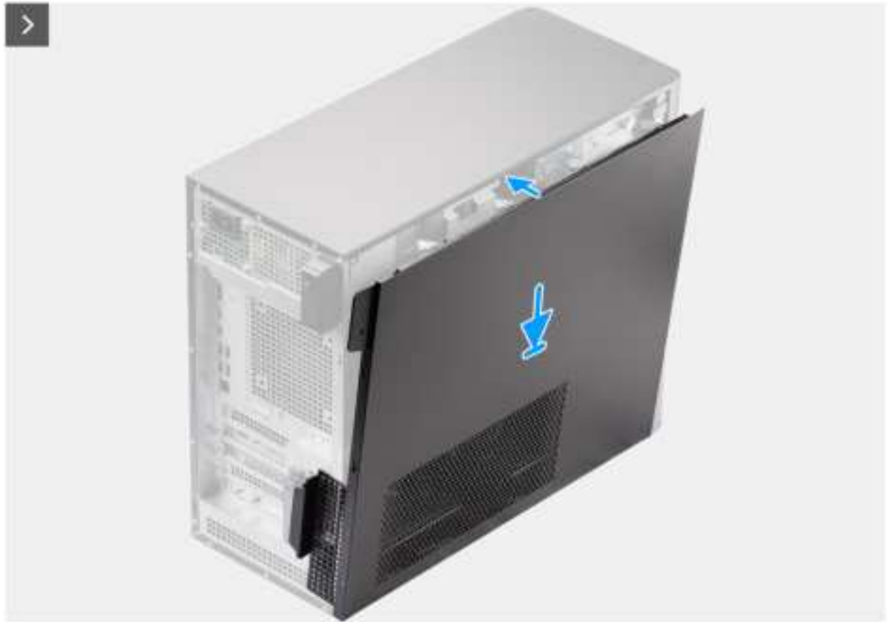
Figure 11. Installing the side cover
