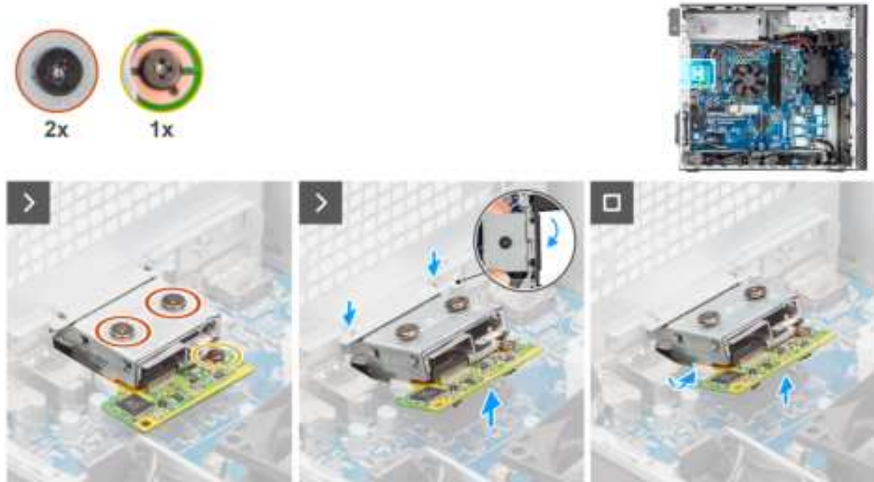
Figure 73. Removing the optional 5GbE Optical module
