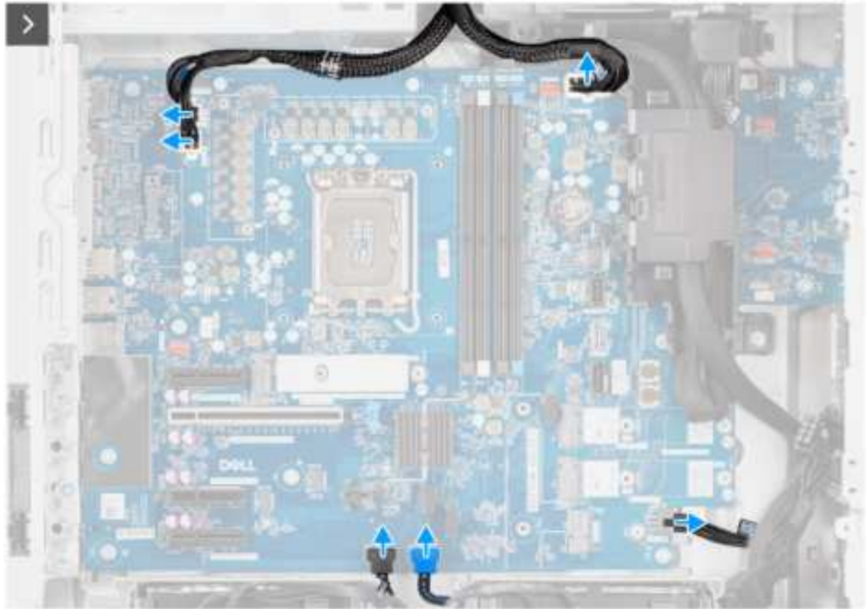
Figure 89. Removing the system board
