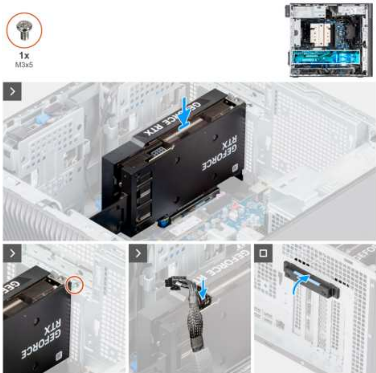
Figure 40. Installing the powered graphics card
