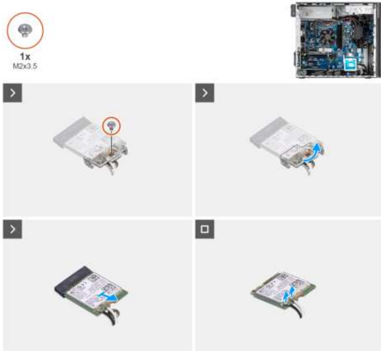
Figure 41. Removing the wireless card
