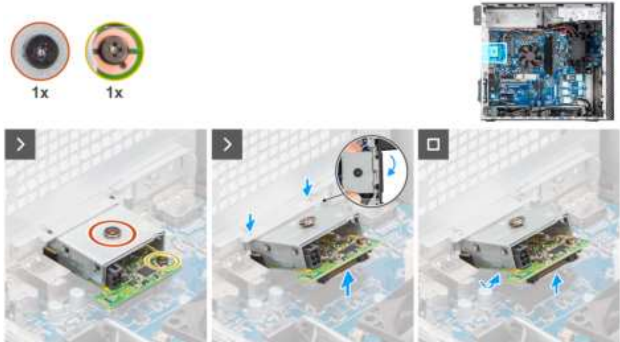
Figure 79. Removing the optional Thunderbolt module
