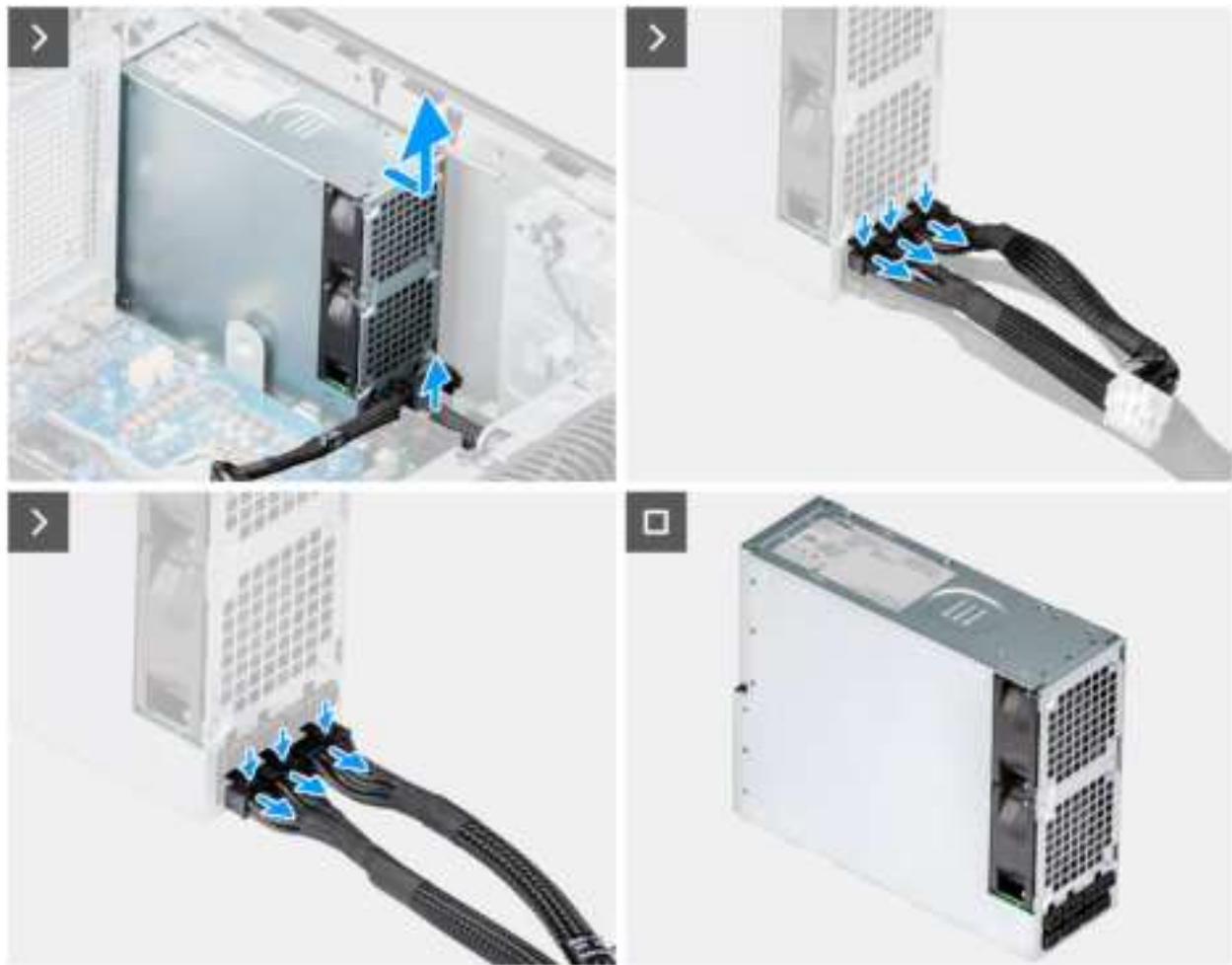
Figure 54. Removing the 1500 W power-supply unit
