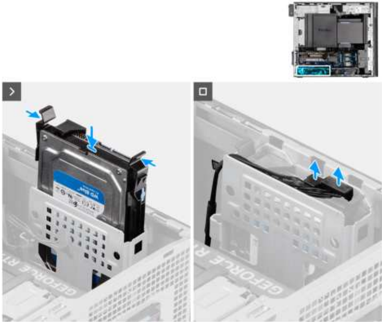
Figure 29. Installing the 3.5-inch hard drive assembly (Bay-2)
