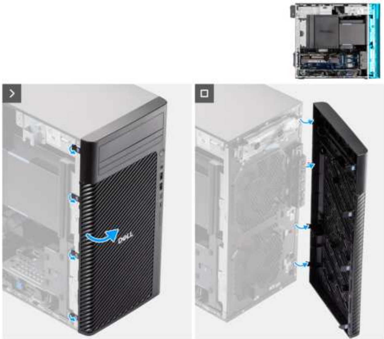
Figure 17. Removing the front bezel
