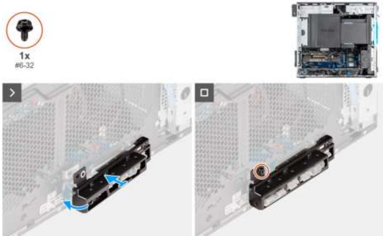
Figure 20. Installing the front I/O bracket
