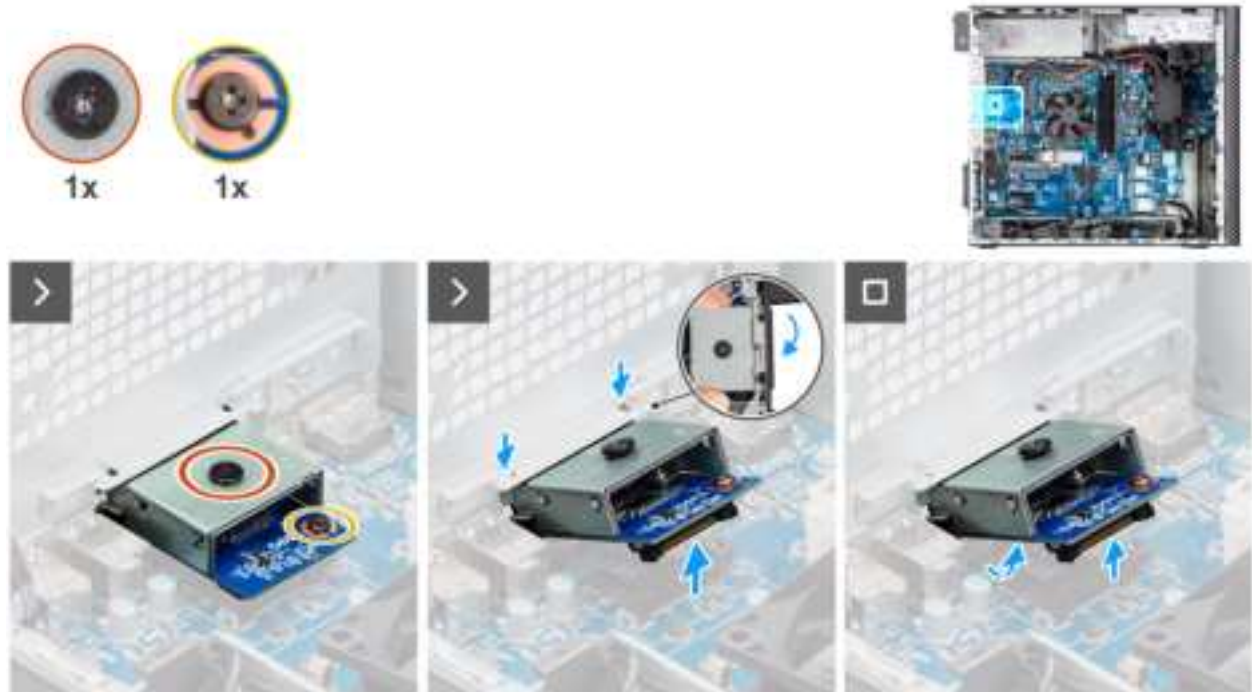
Figure 70. Removing the optional HDMI module
