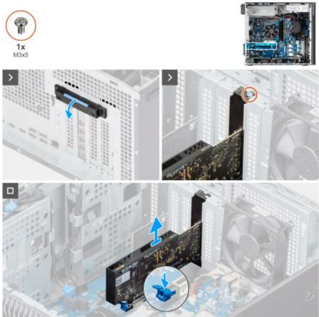
Figure 37. Removing the graphics card
