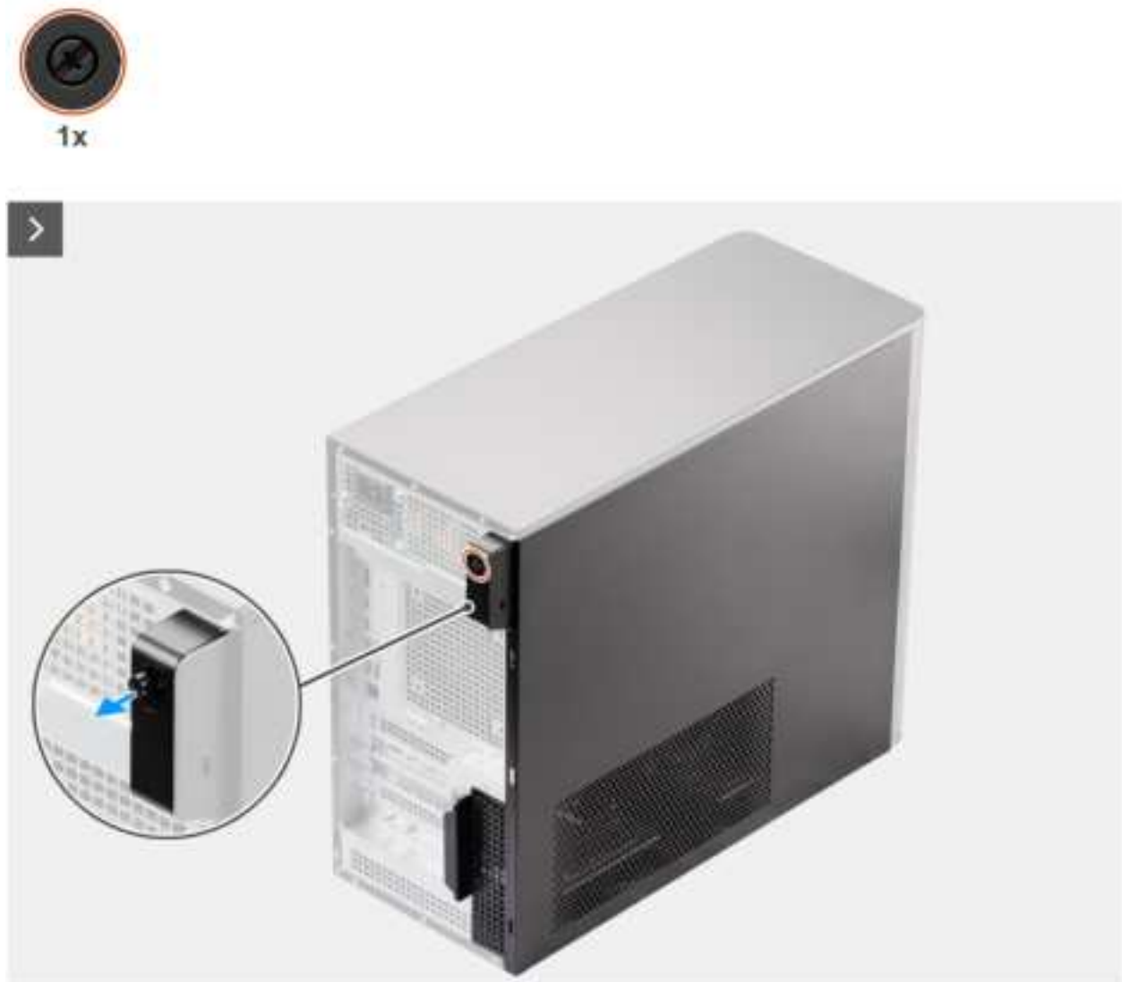
Figure 9. Removing the side cover
