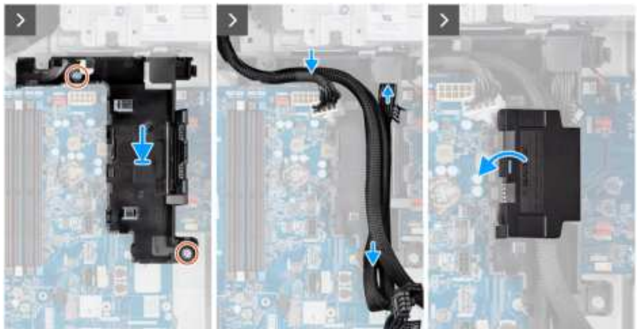
Figure 96. Installing the system board
