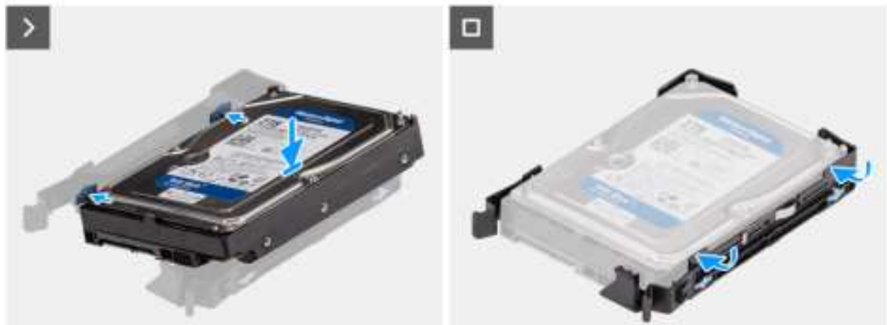
Figure 28. Installing the 3.5-inch hard drive bracket
