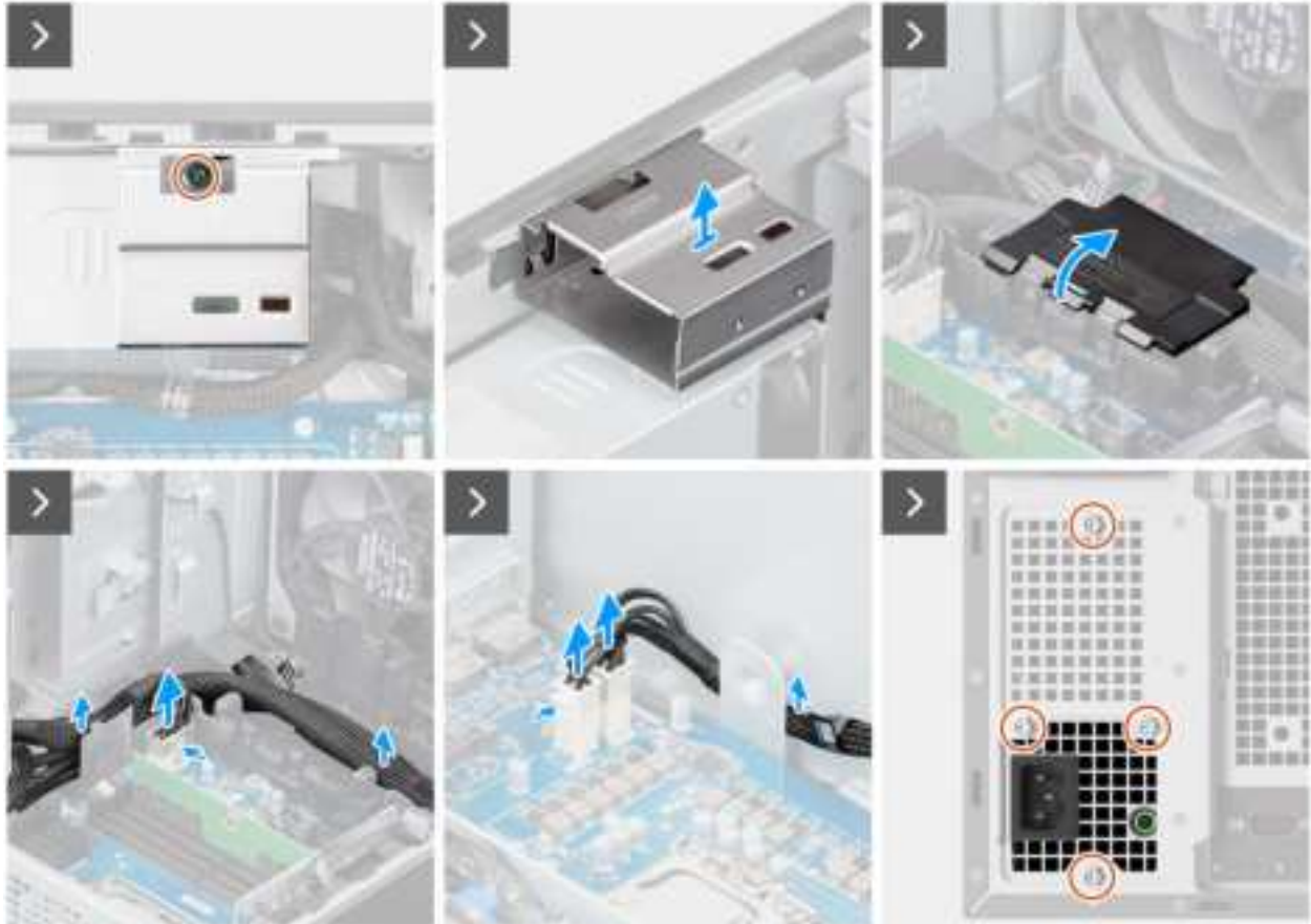
Figure 53. Removing the 1500 W power-supply unit
