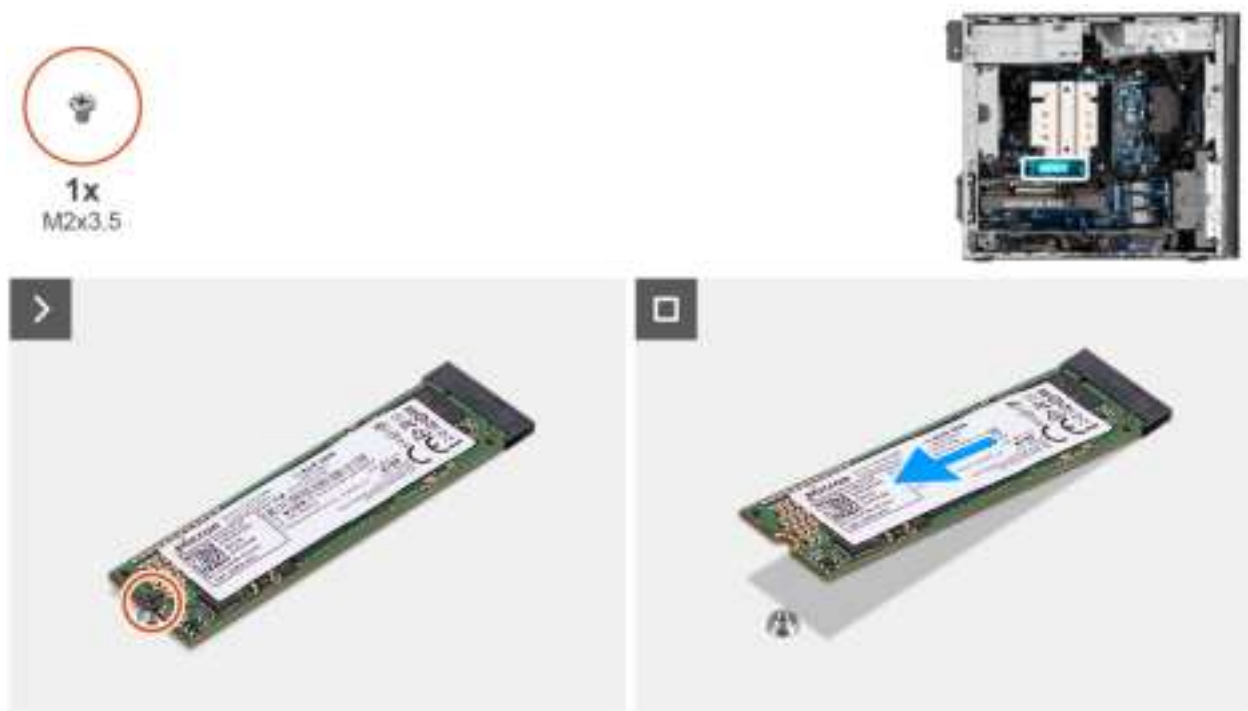
Figure 33. Removing the M.2 2280 PCIe solid state drive
