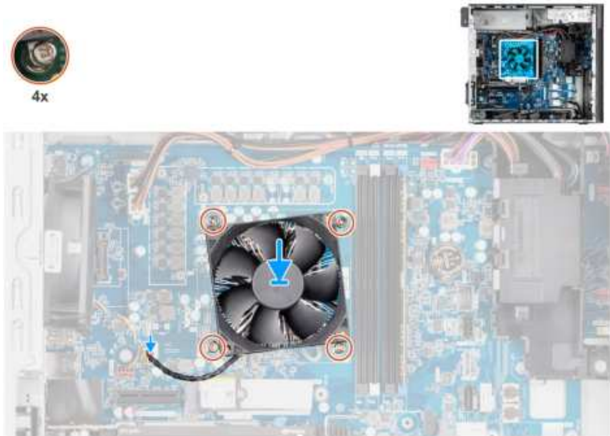
Figure 62. Installing the processor fan and 65 W heat-sink assembly
