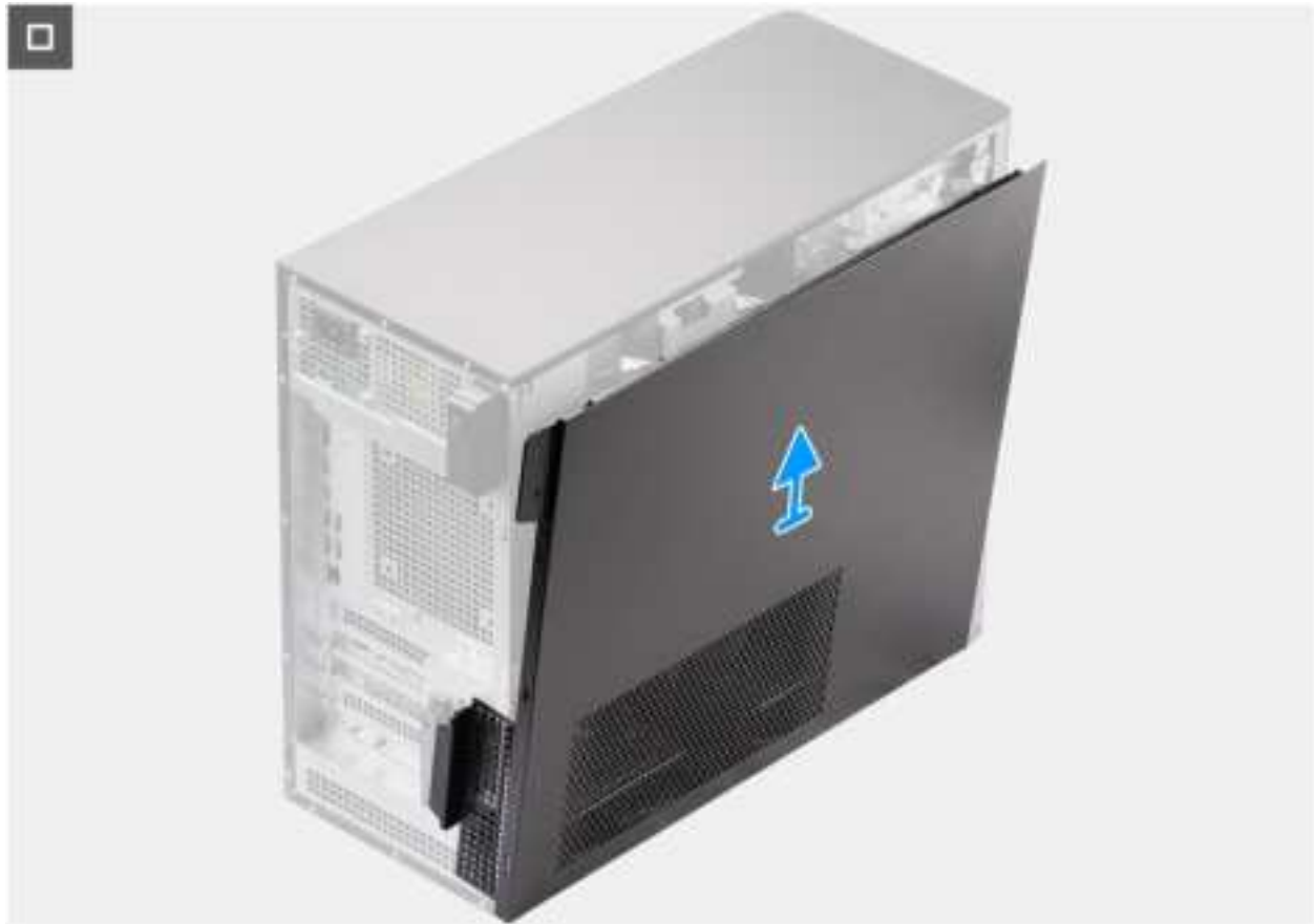
Figure 10. Removing the side cover
