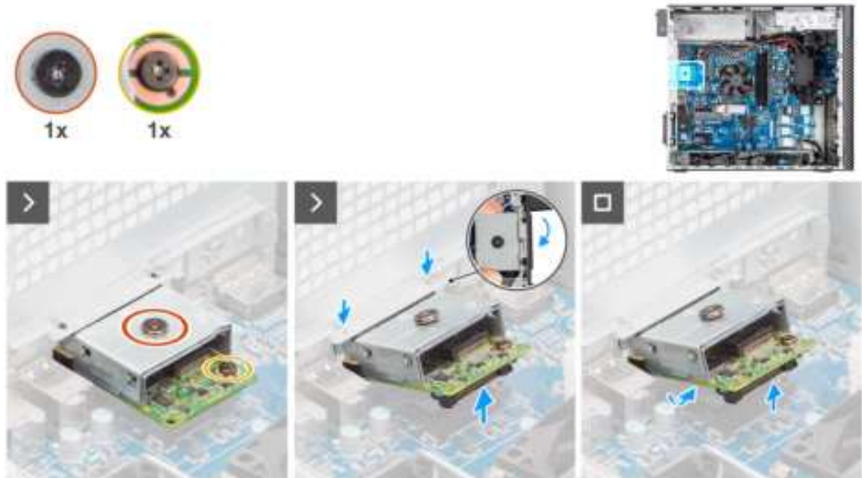
Figure 76. Removing the optional LAN module
