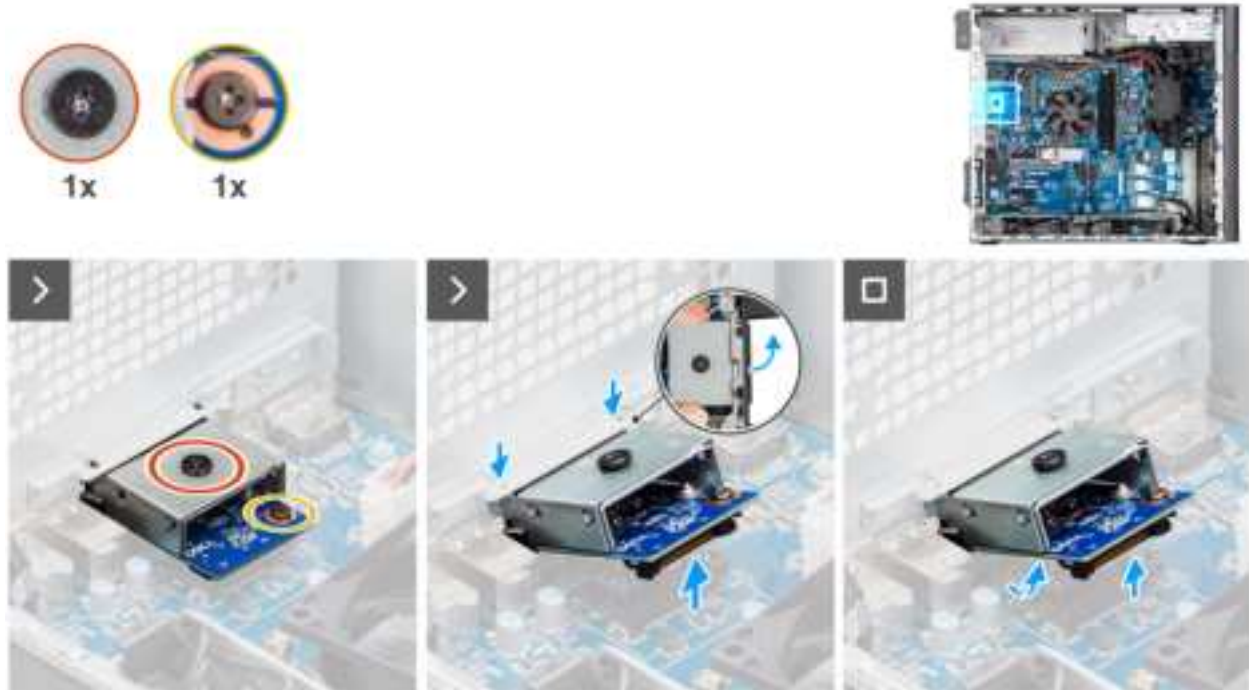
Figure 85. Removing the optional VGA module
