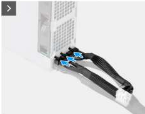
Figure 55. Installing the 1500 W power-supply unit
