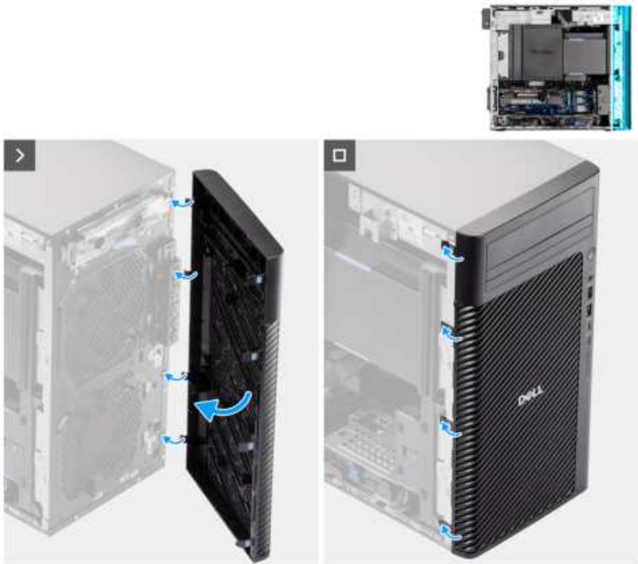
Figure 18. Installing the front bezel
