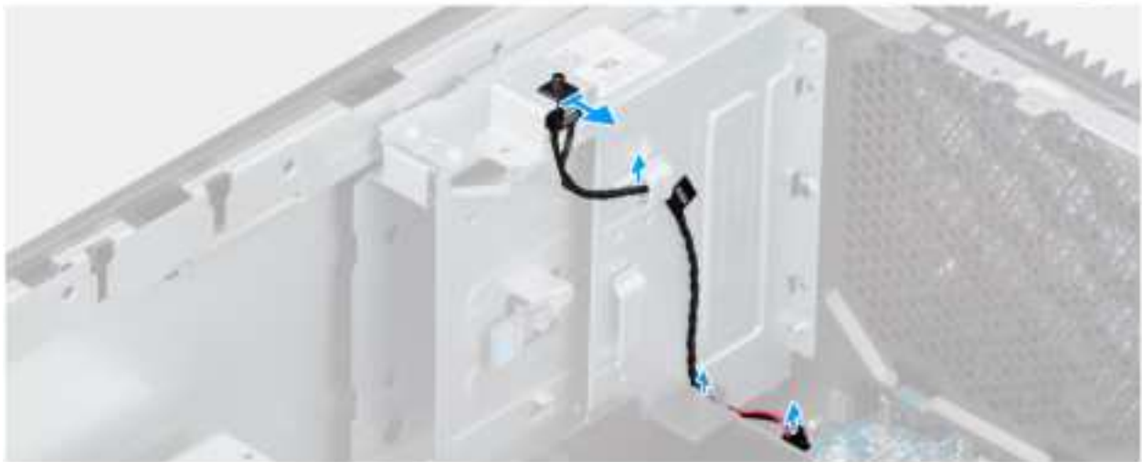
Figure 43. Removing the intrusion switch
