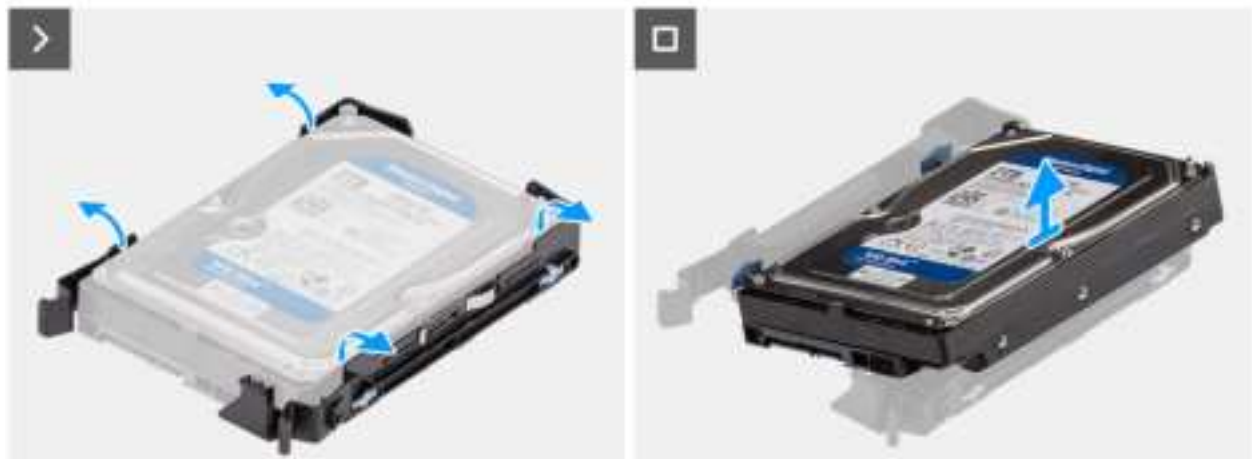
Figure 27. Removing the 3.5-inch hard-disk drive bracket
