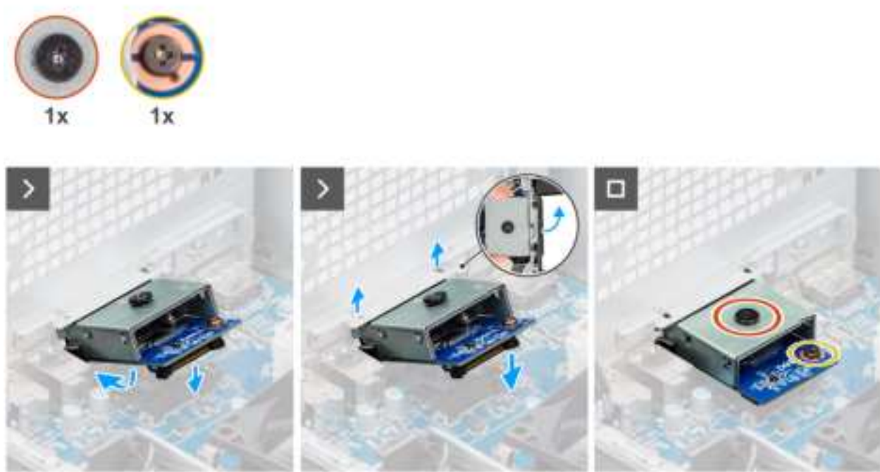
Figure 72. Installing the optional HDMI module
