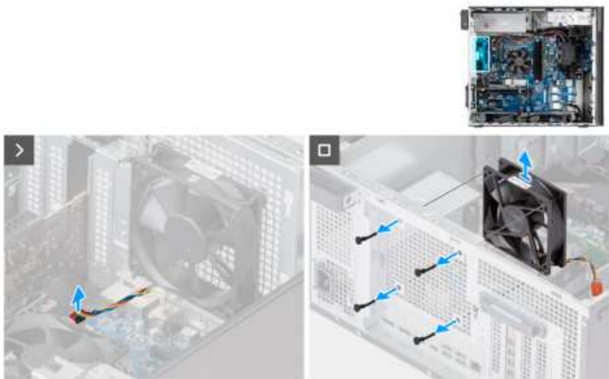
Figure 49. Removing the rear fan for 360 W PSU computers
