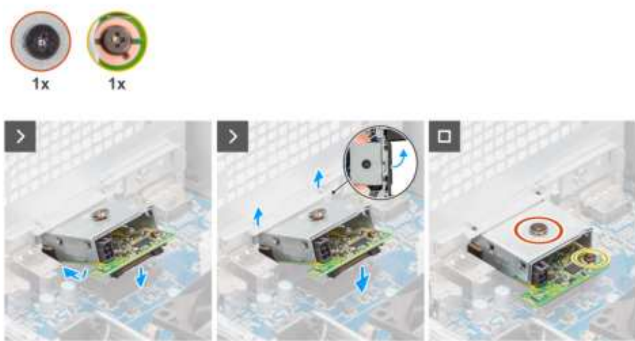
Figure 81. Installing the optional Thunderbolt module
