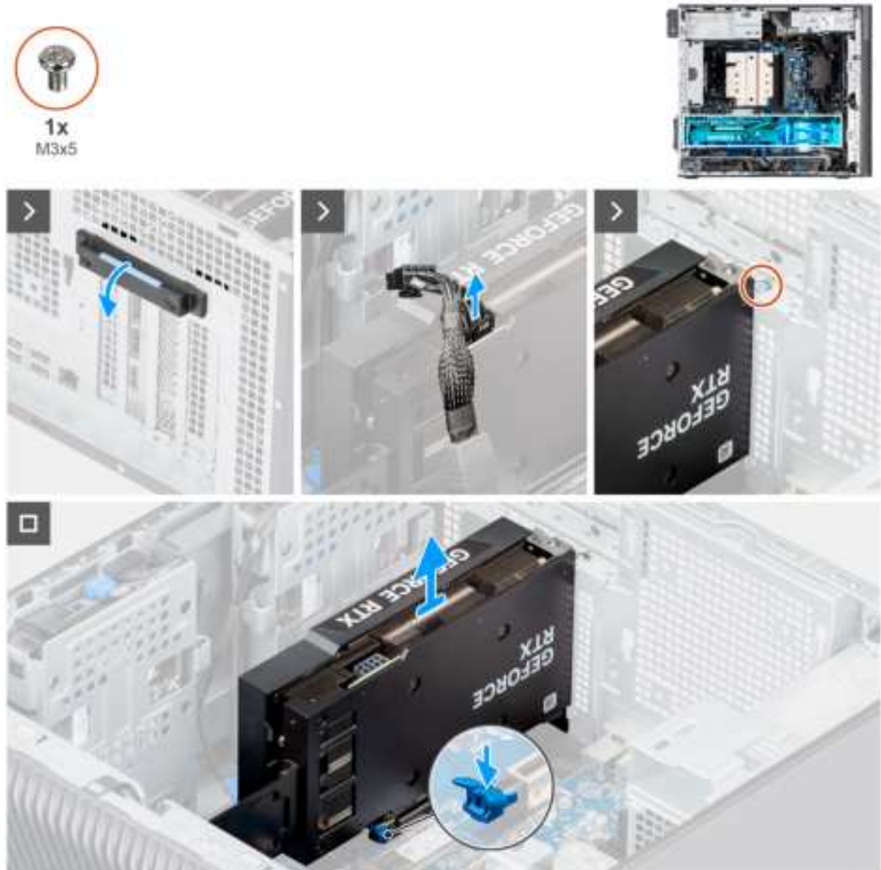
Figure 39. Removing the powered graphics card
