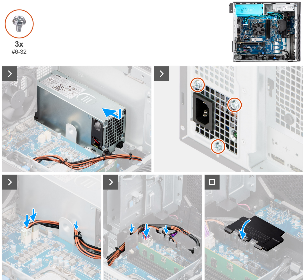
Figure 58. Installing the 360 W power-supply unit
