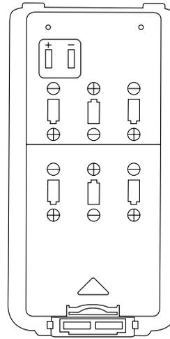
Replace the batteries by following the positive (+) and negative (-) terminal markings inside the case. When the batteries are replaced, replace the battery cover and attach the battery pack to the radio.
