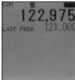
From the example above, the PJ2+ COM is receiving 122.975 MHz with the last frequency being 121.000 MHz. To manually enter a desired frequency such as 118.700 MHz, enter 1 1 8 7 0 0 using the numeric keypad. As each digit is entered, the flashing cursor moves to the next digit. Six digits may be required to select a frequency.
