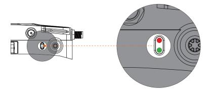
Green LED solid on: Wi-Fi is functioning normally
