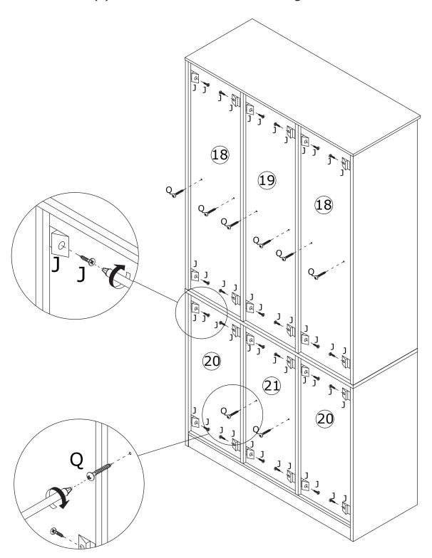
Fix back board 18, 19, 20 and 21 to board 12, 13 and 15 with screw(Q) as shown.
