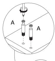
Screw eccentric rod(A) into board 26, 27, 28 and 29 as shown.
