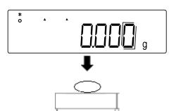
⇒ Place new sample on weighing plate and repeat steps
