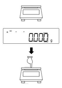
□ Touch slightly the weighing plate to check whether the displayed weighing value in the display is changing
