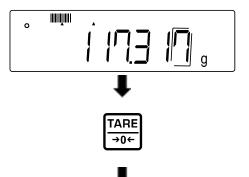
⇒ The weight of the weighing container is shown
