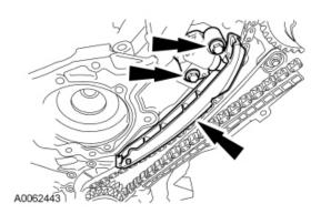
16. Remove the retaining clip from the LH timing chain tensioner.
