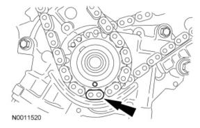
18. **NOTE:** The camshaft phaser and sprocket will be stamped with one of the illustrated timing marks for the RH camshaft.
