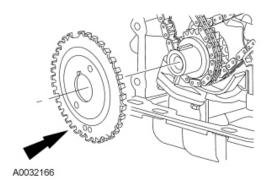
23. **NOTE:** It is necessary to rotate the engine to position the camshaft lobes at base circle to install the roller followers.
