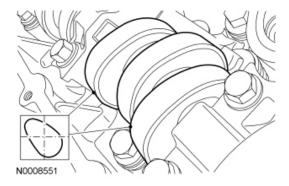
5. *NOTICE:* If the components are to be reinstalled, they must be installed in their original positions. Mark the components for installation into their original locations. Failure to follow these instructions may result in engine damage.
