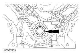
10. Remove the bolts, the LH timing chain tensioner and tensioner arm.
