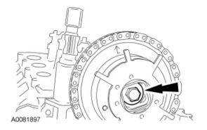
4. *NOTICE:* Damage to the camshaft phaser sprocket assembly will occur if mishandled or used as a lifting or leveraging device.
