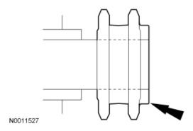
6. Rotate the crankshaft to position the crankshaft sprocket timing mark in the 6 o'clock position.
