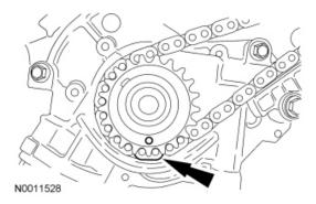
14. NOTE: Make sure the upper half of the timing chain is below the tensioner arm dowel.
