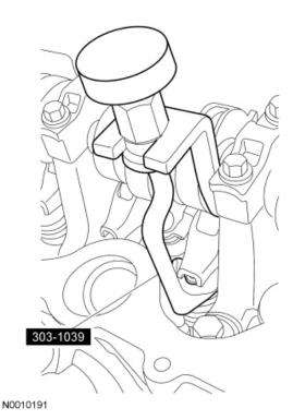
9. *NOTICE:* The crankshaft cannot be moved past the 6 o'clock position once set or engine damage may occur.
