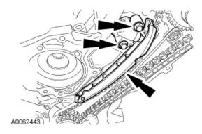
11. Remove the bolts, the RH timing chain tensioner and tensioner arm.
