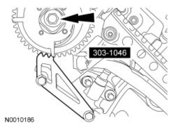
15. NOTICE: Damage to the camshaft phaser sprocket assembly will occur if mishandled or used as a lifting or leveraging device.
