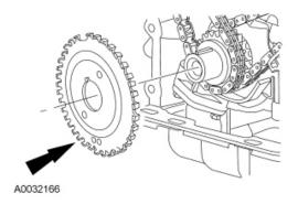
3. Position the crankshaft keyway at the 12 o'clock position.
