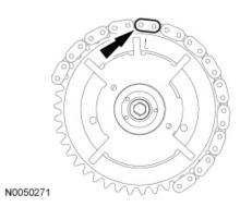
15. **NOTE:** The LH timing chain tensioner arm has a bump near the dowel hole for identification.
