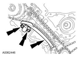
20. Remove the retaining clip from the RH timing chain tensioner.
