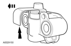
21. **NOTE:** The RH and LH camshaft phaser sprockets are similar. Refer to the single timing mark to identify the RH camshaft phaser sprocket and the L timing mark to identify the LH camshaft phaser sprocket.
