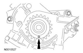
7. NOTICE: If one or both of the tensioner mounting bolts are loosened or removed, the tensioner sealing bead must be inspected for seal integrity. If cracks, tears, separation from the tensioner
