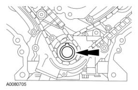
4. **NOTE:** If the camshaft lobes are not exactly positioned as shown, the crankshaft will require one full additional rotation to 12 o'clock.
