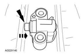
9. Install a retaining clip on the tensioner to hold the plunger in during installation.
