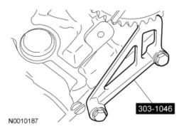
5. Install the crankshaft sprocket, making sure the flange faces forward.
