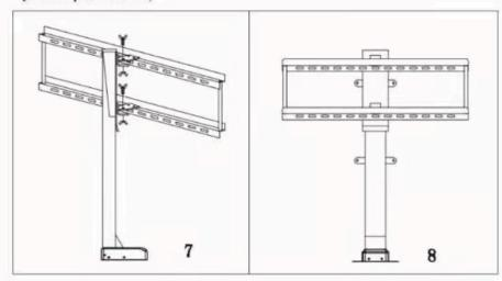
Install TV bracket (vertical) on the back of the TV with bolt.
