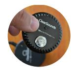
**STEP 1:** Remove the top of the QUATTRO 4 (BT4 Removable Mic).
