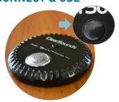
STEP 1: Place BT4 Removable Mic in a position that best captures the voice(s) that you want to hear. On the BT4 Removable Mic, BRIEFLY press BUTTON on the Mic and the device will begin connecting to the QUATTRO 4.
