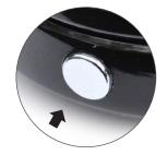
**STEP 1:** Ensure QUATTRO 4 is turned off, press and hold multi-function button for approximately six seconds.
