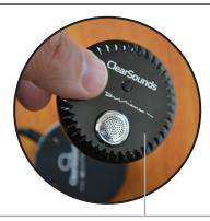
BT4 Removable Bluetooth Mic: This entire disc is the removable mic. It magnetically connects to the main base. When charging the Quattro 4.0, make sure to have the mic connected as this is how the mic charges.
