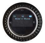
**STEP 4:** When the device name appears on the QUATTRO 4 screen, it is paired and connected.
