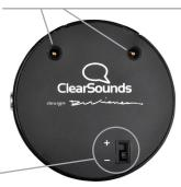
Battery Engage Switches: There is a battery engage switch on both the removable mic and the Base. This switch MUST be in the + position on both the Mic & Base for the unit to function. By switching to the  $\overline{\phantom{a}}$  position, the battery is disengaged from the circuit. This switch does NOT need to be put in the - position. The purpose is to protect the integrity of the battery when stored in the warehouse.
