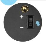
**STEP 1:** Use the tip of a pen to move both battery engagement +/- switches into the + position on the QUATTRO 4 and BT4 Removable Mic. **Do NOT turn them off!**
