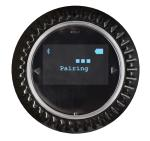
**STEP 2:** After around six seconds, the QUATTRO 4 announces Pairing, and Pairing... appears on the QUATTRO 4 screen.
