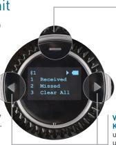
TFK Touch Function Kev: The touch sensor is used to answer & end phone calls. It activates the LCD screen to view. It pauses & plays music. Tap twice to active the voice control for the second device
