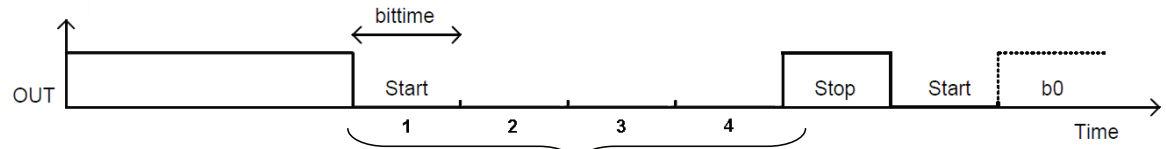
Synchronization pulse (start (0)x4bits + stop (1)x1bit)
