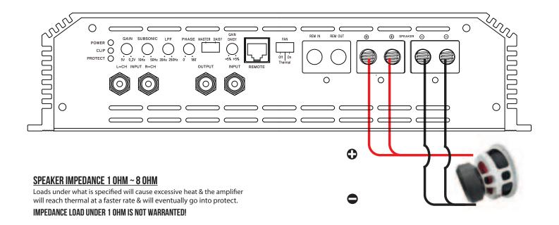
We recommend using minumum 8 Ga speaker cables to acquire the intended performance & efficiency. Run the speaker cables from your speakers to the amplifier's mounting location.
