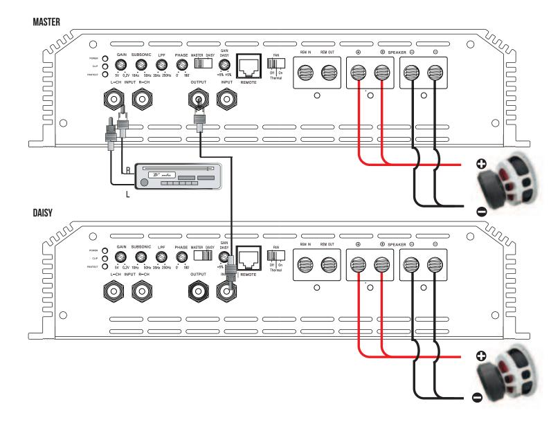
In daisy chain mode, the master amplifier's audio settings, such as gain, crossover, etc., are routed to the amplifier marked as daisy. From that daisy amplifier, you can route the input signal from the master amplifier to a second daisy by using the output RCA on the first daisy amplifier. You can continue adding amplifiers in a chain this way.
