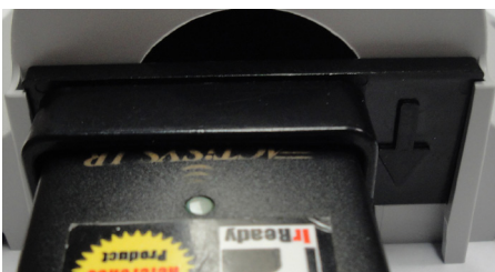
Figure 23: IR programming bracket inserted into the adapter rails
