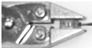
Figure 8: Compress the gel cap
