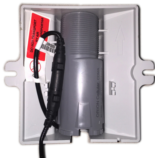
Figure 20: Cable position with Nicor connector
