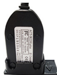
Optical head inserted into bracket
