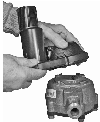
Figure 38: Remove assembly from meter
