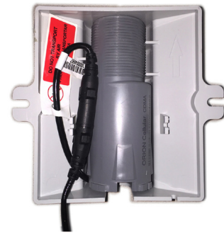
Figure 5: Endpoint with Nicor connection in remote enclosure box
