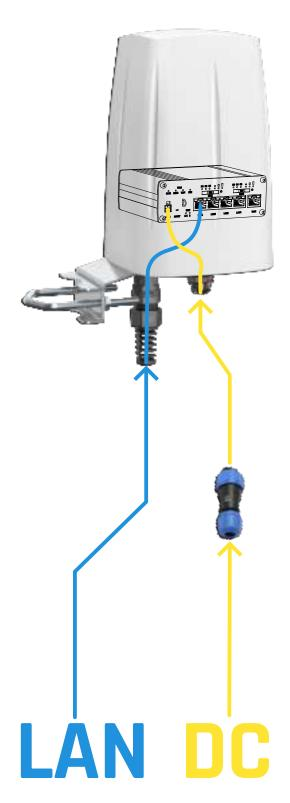
Please note that for Teltonika RUTX series, the DC power source ranges from 9 to 50 VDC, while for the RUT series it is 9 to 30 VDC.
