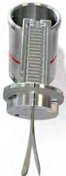
Sample container with swab to be used in ion-scanners.
