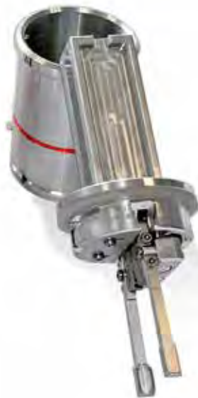
Sample container with automatic grasp for picking various objects.
