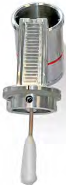
Sample container using a cotton bud for taking liquids.
