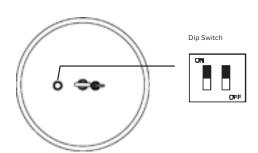
3. Adjust the lighting level to your desired lumen output using the lumen select switches. If you're using the default output, disregard this step.
