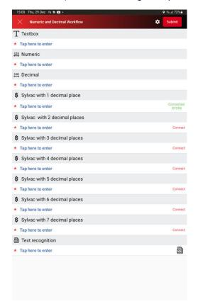
c. If user change the focus to another Sylvac widget and device is already connected then status of focused widget is getting changed from "Connect" to "Connected SY295". Device will be attached to that widget.
