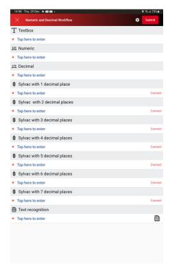
ii. Tap on "Connect" button it will redirect to another screen where it will scan the available BLE devices and listing all the devices with name and address. Select Sylvac device of your choice (Most probably its name starts with "SY" e.g., SY295)
