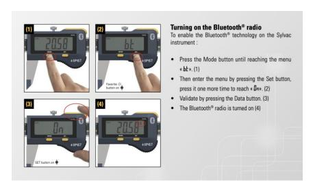
Note: If Bluetooth Symbol is blinking that means it is ready to connect and after connected with any device it will be stop blinking and be steady there.
