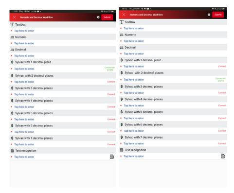
14. Once Device is connected, user can take measurement and can push the Sylvac's device measurement via tapping Data button easily. Measurement/Reading sent by device will be display in focused widget with device attached.
