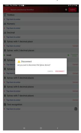
17. After disconnecting the device, User can connect to another device of same device by following the connection step. (From step 13.)
