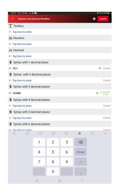
15. Sylvac widget have properties like Minimum number, low limit, high limit, Maximum number, decimal places same as Decimal widget and also behave or act similar to Decimal widget. Sylvac widget is support 0 up 7 decimal places. After putting the measurement or read value to the Sylvac widget, Sylvac widget will display the result based on the properties like minimum number, higher limit, low limit, maximum number, decimal places. Please refer the below images and table to see how it behaves.
