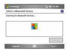
Start a scan on the controller. On a Trimble Tablet, Tap [Add a device]. On a TSC2 controller, tap the [devices] tab and tap. [New Partnership...]. On a Trimble CU (Model 3) controller, tap the [scan device] tab and then tap [scan]. On a Trimble CU controller, tap [Scan Device]. (Do not use [stop] - wait for the scan to complete).
