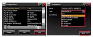
>>>Next 3 Times the Perirals set up button will be available | Also remember to use the correct driver for the depth sounder if driver not available select generic NMEA and the port information default is Bluetooth but serial is incorraged
